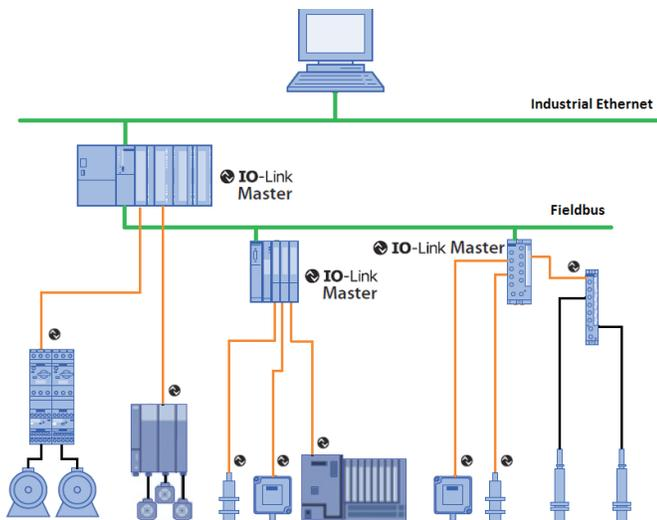
Figure 5. IO-Link Compatibility with Existing Industry Protocols
