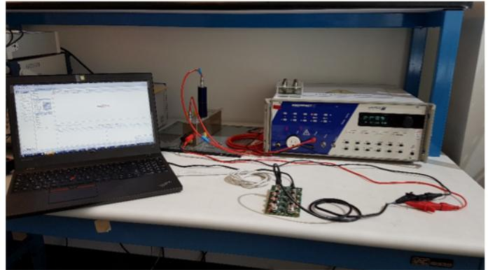
Figure 28. EFT Burst and Surge Testing of MAX14819
