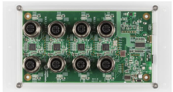
Figure 23. MAXREFDES145 8-Port IO-Link Master Reference Design
