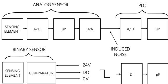
Figure 1. Evolution of Sensors from Analog to Binary
