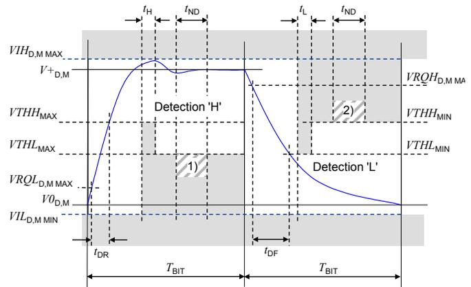
NOTE In the figure, 1) = no detection 'L'; and 2) = no detection 'H'
