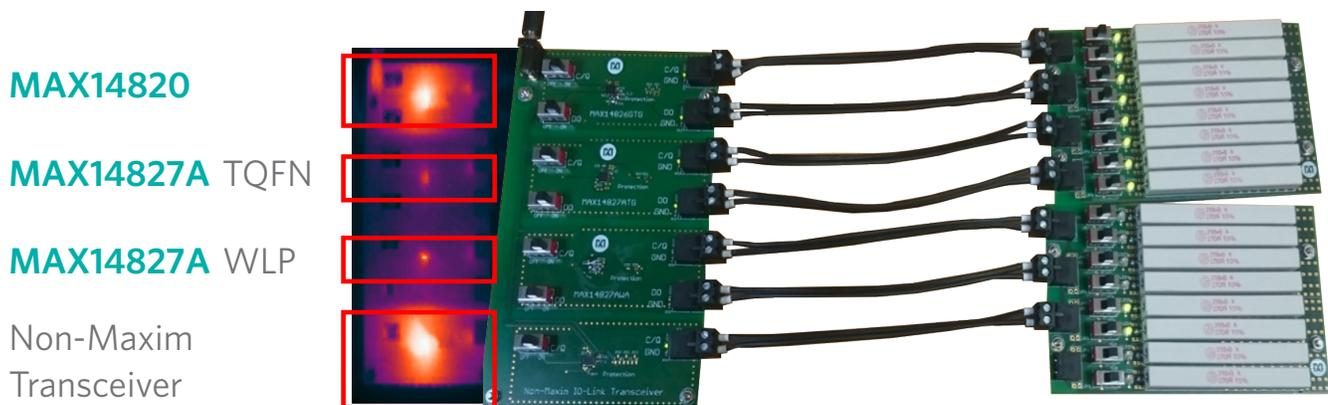
Figure 27. Comparison of Transceiver Power Dissipation at Full Load, Relative to Competitive Device
