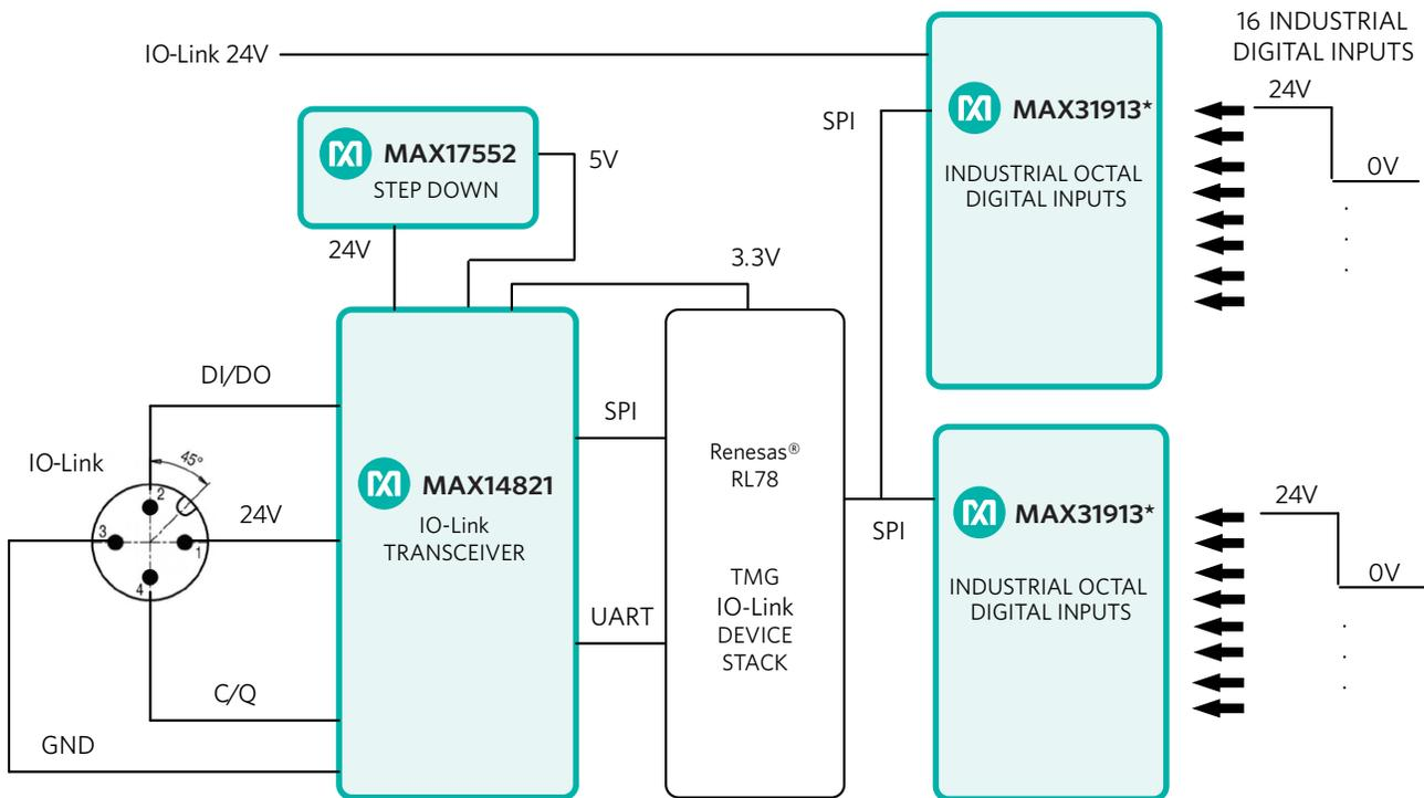
Figure 21. MAXREFDES36 Digital Input Hub Block Diagram
