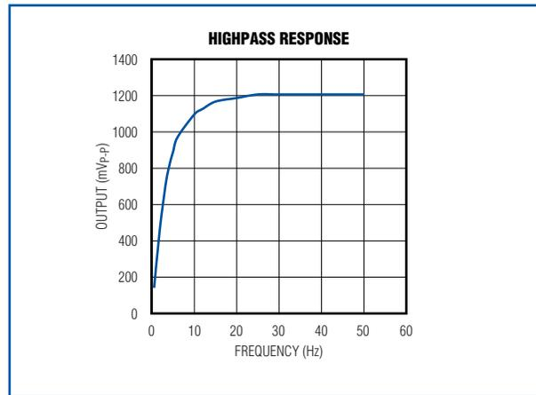
Figure 4. Frequency response is shown for an AC-coupled video connection with 220µF capacitor.
