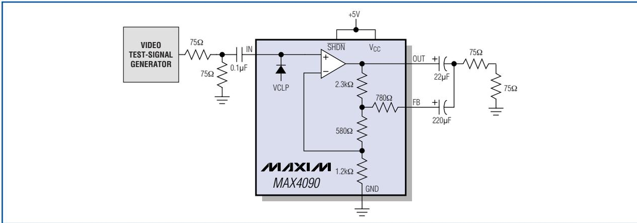
Figure 5. The MAX4090 video driver includes SAG compensation.
