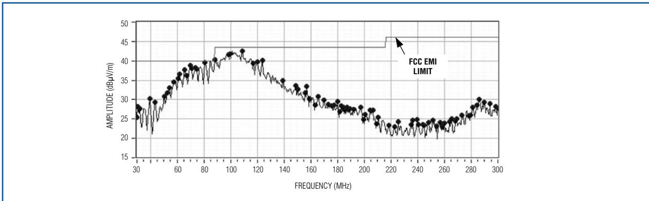
Figure 8. The MAX9705 radiated emissions data is shown for a 24in, unshielded twisted pair in spread-spectrum modulation mode.
