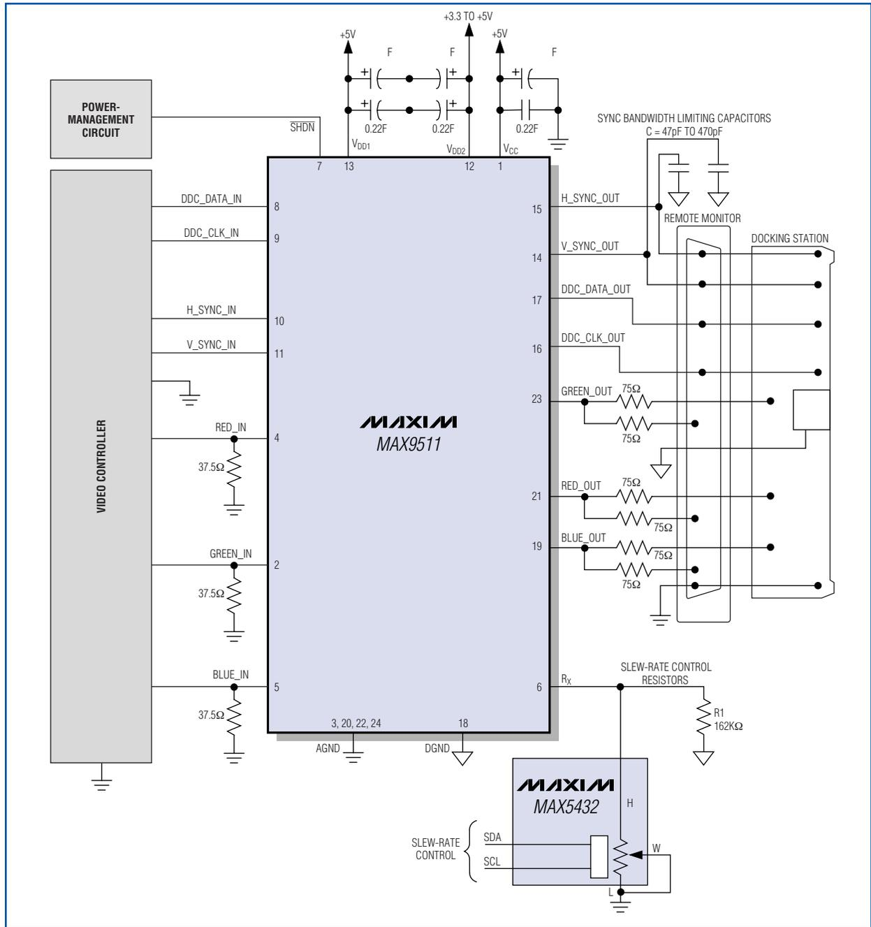
Figure 4. The MAX9511 drives multiple outputs. Adjustable filtering is controlled by the MAX5432 I<sup>2</sup>C-adjustable digital potentiometer.
