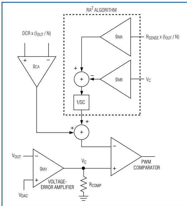
Figure 5. The RA<sup>2</sup> algorithm is implemented.
