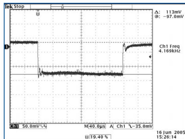
Figure 7. Peak current-mode transient response is shown for the MAX8810A.
