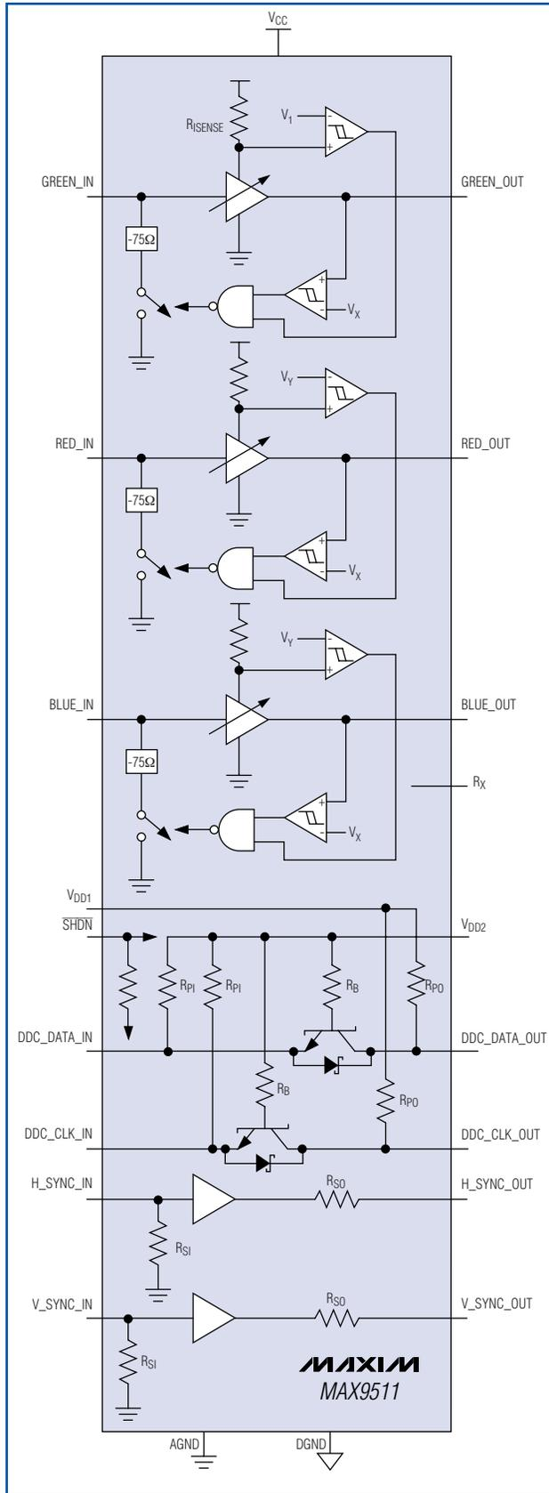
Figure 3. The MAX9511 VGA interface has EMI suppression.
