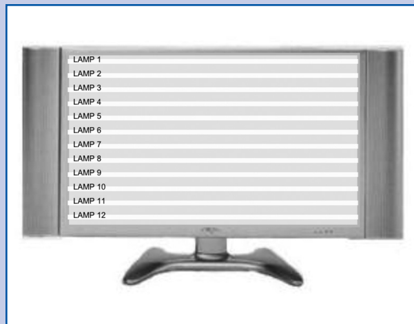
Figure 12. LCD TVs contain from 4 to 40 CCFLs.
