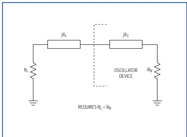
Figure 4. Reflection amplifier model
