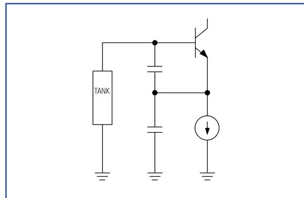
Figure 1. The basic Colpitts oscillator
