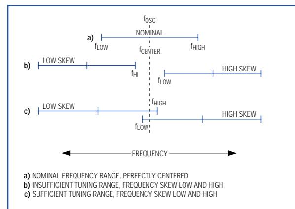
Figure 5. Tuning range and frequency shifts
