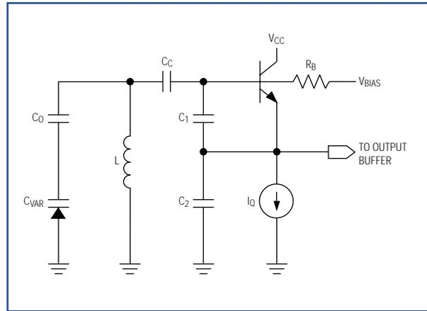
Figure 2. Use of the Colpitts topology in a VCO
