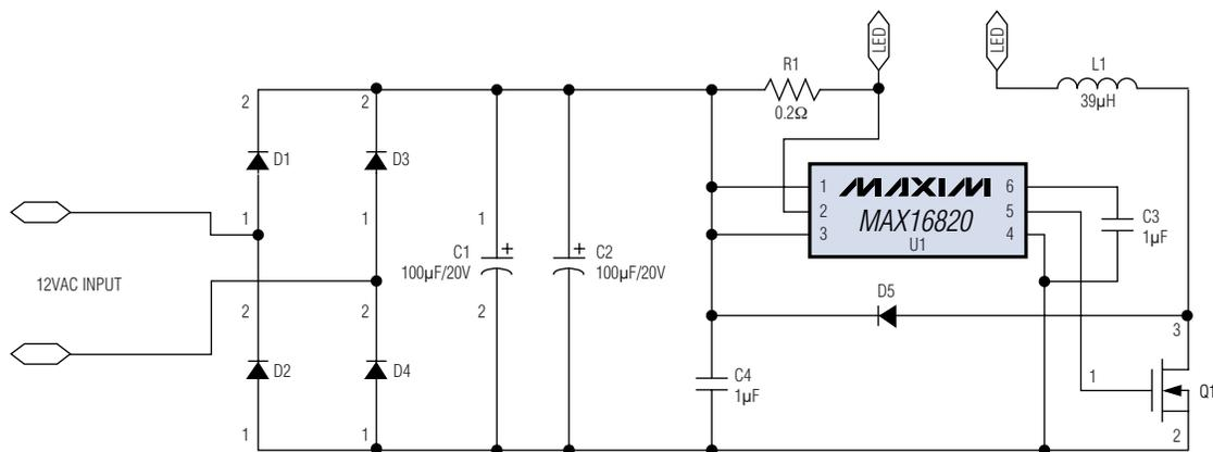
The 5W MR16 LED lamp circuit is shown using the MAX16820 LED driver. The LEDs shown are the LedEngin 5W WLEDs. (See page 10.)
