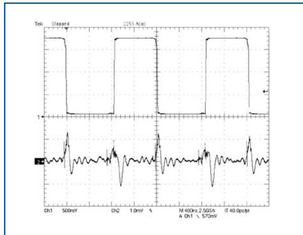
Figure 7. The MAX9509's output (bottom trace) is measured vs. time, taken with respect to a 1V<sub>p-p</sub> video signal. The spikes are 1.4mV<sub>p-p</sub>. The top trace is the voltage on the top plate of the charge pump's flying capacitor.
