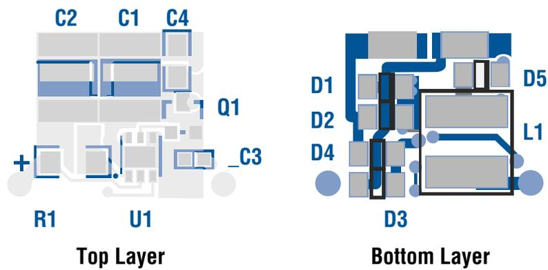
Figure 7. The LED+ and LED- DC-output connection pads can be seen on the 5W MR16 LED lamp driver PCB silk screen (top and bottom layers).
