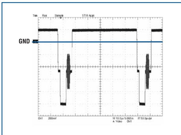
Figure 3a. The OPA360's output waveform contains a blue line indicating the approximate DC average of a 50% flat-field signal.
