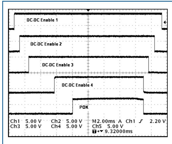
*Figure 2. Beginning with DC-DC converter 1, the circuit of Figure 1 switches on three additional converters in sequence and generates a POK signal. Pulling the circuit's on/off input low removes the POK signal and switches off all four converters in reverse order.*
