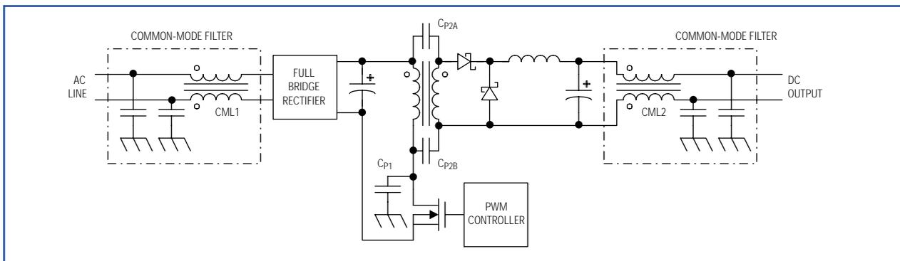
*Figure 7. Common-mode filters in this typical off-line power supply reduce noise common to both sides of the input and output.*
