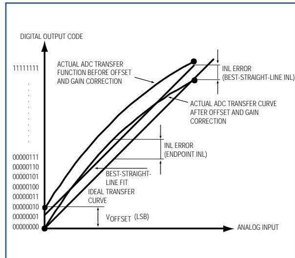
Figure 1b. Best-straight-line and endpoint fit are two possible ways to define the linearity characteristic of an ADC.
