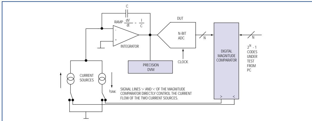
Figure 2. This circuit configuration is an analog integrating servo loop.
