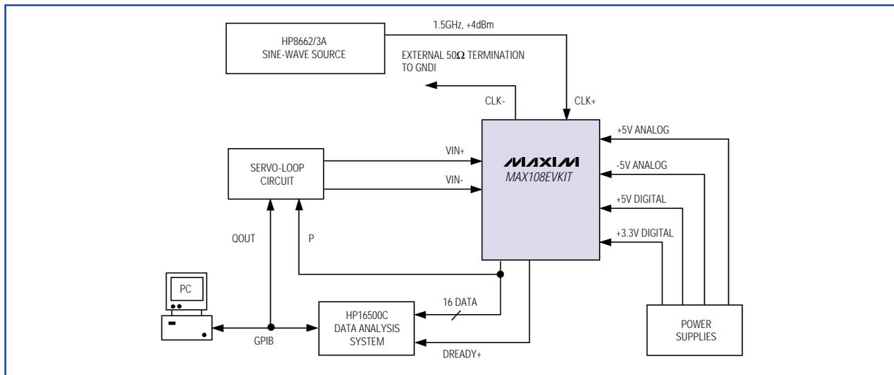
Figure 3. With the aid of the MAX108EVALKIT and an analog integrating servo loop, this test setup determines the MAX108's INL and DNL characteristics.
