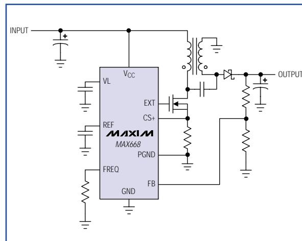
Figure 5. Otherwise similar to a flyback regulator, the SEPIC has continuous primary and secondary currents that generate less noise.
