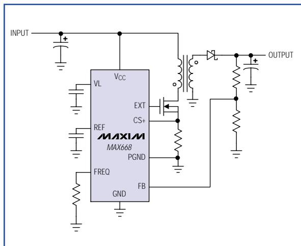
Figure 4. A flyback regulator maintains regulation for inputs that range above and below the output voltage.
