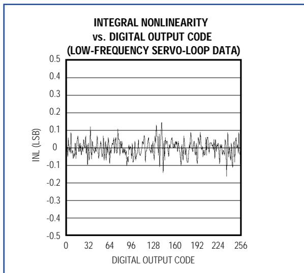
Figure 4a. This plot shows typical INL for the MAX108 ADC, captured with the analog integrating servo loop.
