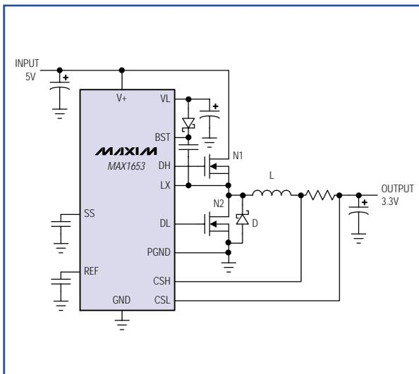
Figure 1. This illustrative step-down switching regulator features an external switching transistor (N1) and synchronous rectifier (N2).
