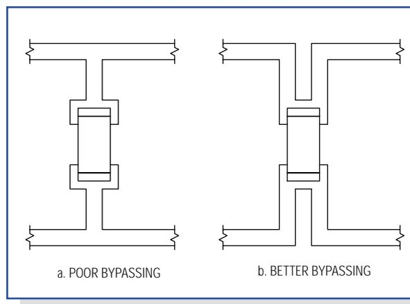
*Figure 12. Poor bypass connections (a) add trace inductance and resistance to the capacitor. In the better connection (b), trace parasitics add to the capacitor’s filter action.*
