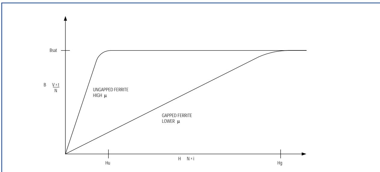
Figure 9. Gapping a ferrite core forces magnetic flux out of the core and allows the inductor or transformer to store energy in a field surrounding the device.
