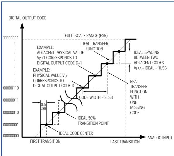
Figure 1a. To guarantee no missing codes and a monotonic transfer function, an ADC's DNL must be  $\leq 1$ LSB.
