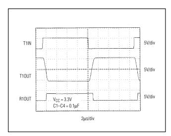
Figure 7. MAX3385E Loopback Test Result at 120kbps
