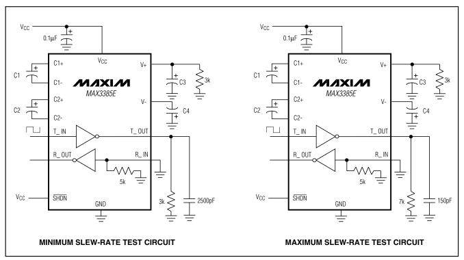
Figure 1. Slew-Rate Test Circuits
