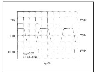
Figure 8. MAX3385E Loopback Test Result at 250kbps
