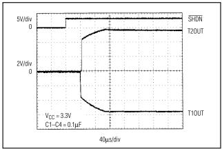
Figure 2. Transmitter Outputs Exiting Shutdown or Powering Up
