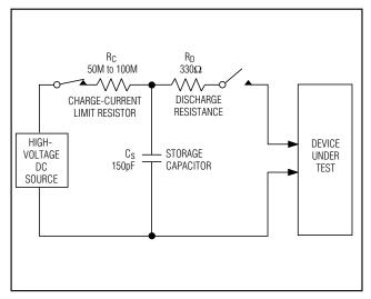
Figure 4a. IEC 1000-4-2 ESD Test Model
