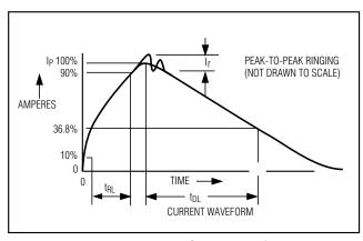
Figure 3b. Human Body Model Current Waveform
