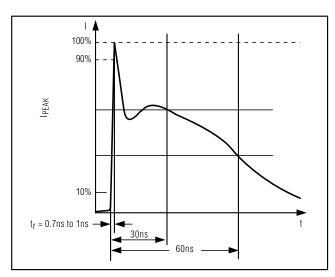
Figure 4b. IEC 10000-4-2 ESD Generator Current Waveform
