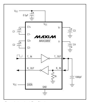
Figure 6. Loopback Test Circuit
