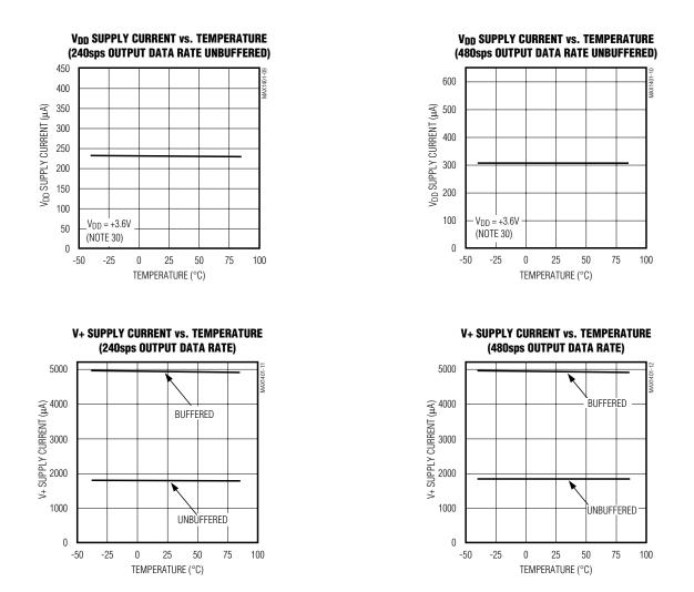
**Note 30:** Minimize capacitive loading at CLKOUT for lowest V<sub>DD</sub> supply current. *Typical Operating Characteristics* show V<sub>DD</sub> current with CLKOUT loaded by 120pF.
