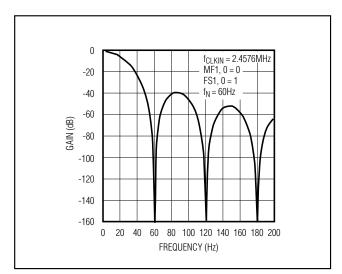
Figure 10. Frequency Response of the SINC<sup>3</sup> Filter (Notch at 60Hz)
