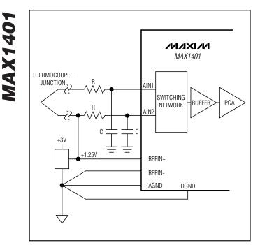
Figure 15. Thermocouple Application with MAX1401
