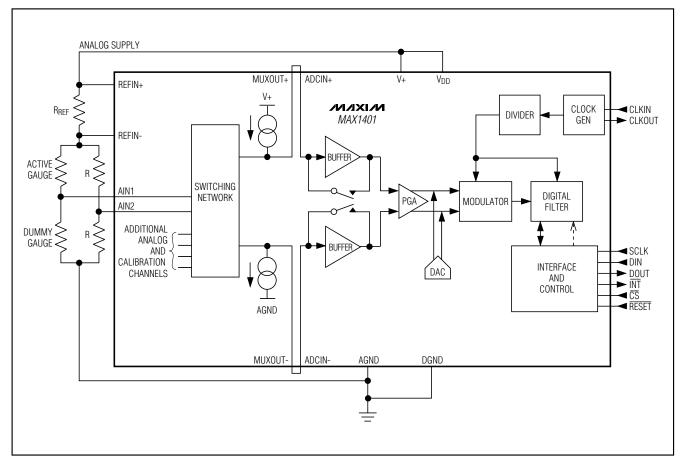
Figure 14. Strain-Gauge Application with MAX1401
