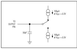
Figure 1. Load Circuit for Bus-Relinquish Time and  $V_{OL}$  and  $V_{OH}$  Levels
