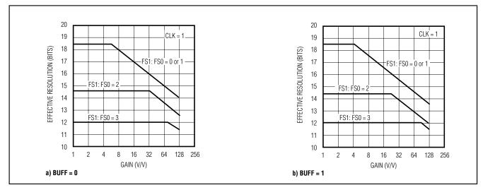
Figure 7. Effective Resolution vs. Gain and Notch Frequency
