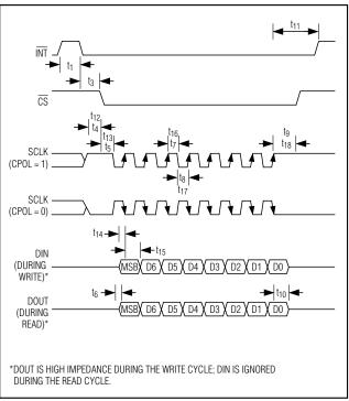
Figure 4. Serial-Interface Timing
