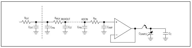
Figure 6. Analog Input, Buffered Mode (BUFF = 1)
