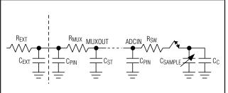
Figure 5. Analog Input, Unbuffered Mode (BUFF = 0)
