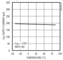
**V+ SUPPLY CURRENT vs. TEMPERATURE** (120sps OUTPUT DATA RATE)
