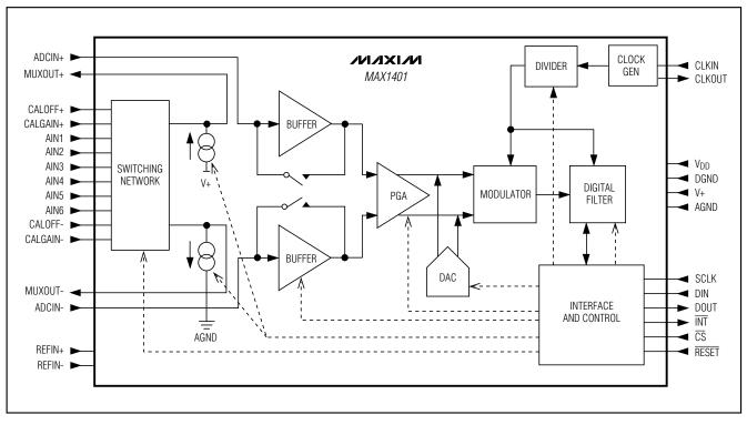
Figure 2. Functional Diagram
