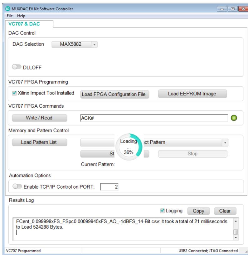
Figure 9. Pattern load in progress.
