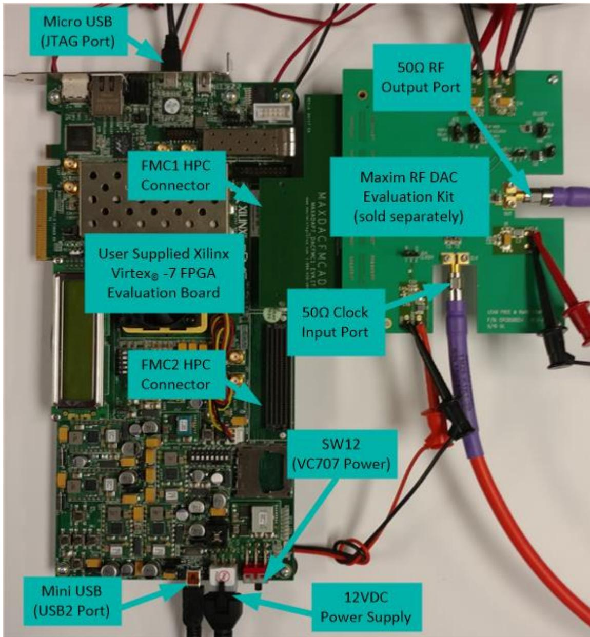
Figure 43. Hardware setup using the VC707 FPGA board and the MAX5882 EV kit.
