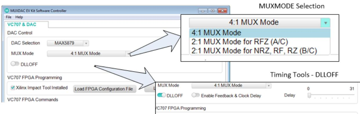
Figure 6. MAX5879 MUX mode and timing controls.
