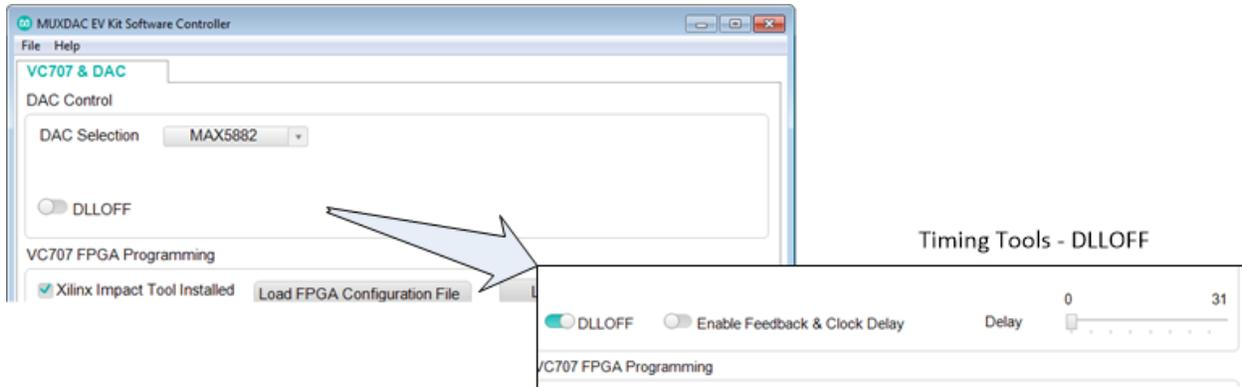
Figure 7. MAX5882 timing controls.
