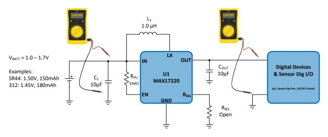
Figure 22. Digital 1.8VDC MAX17220 SMPS Circuit for Wearable Medical/Healthcare Applications
