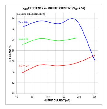
Figure 52. Efficiency of the Analog 5V MAX77642 SMPS Circuit
