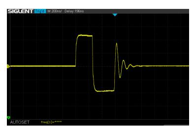
Figure 8. Typical MAX38640A VLX Waveform with Light Load
