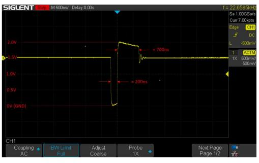
Figure 28: Typical MAX17220 V<sub>LX</sub> Waveform with 2mA Load
