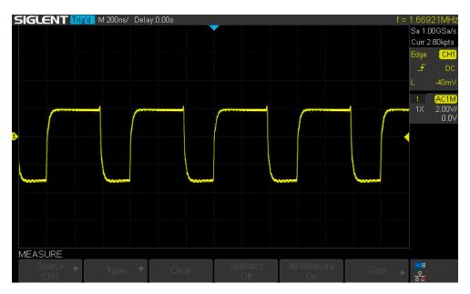
Figure 40. Typical MAX20343H HVLX Waveform with 246mA Load
