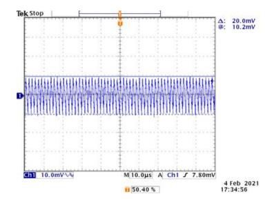
Figure 36. Typical Output Ripple Voltage ( $V_{IN}$  = 4.2VDC,  $I_S$  = 100mA)
