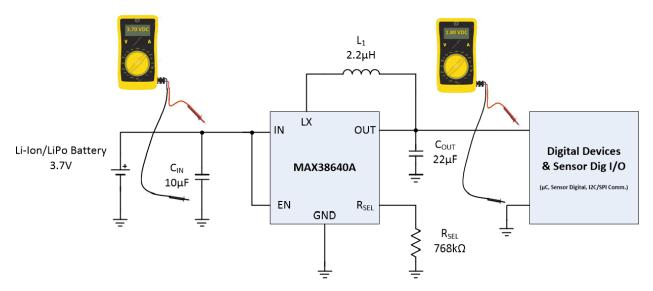
Figure 12. Digital 1.8VDC MAX38640A SMPS Circuit for Wearable Medical/Healthcare Applications
