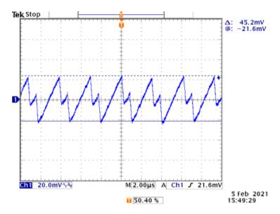
Figure 53. Typical Out Ripple Characteristic (V<sub>IN</sub> = 4.2VDC, I<sub>S</sub> = 100mA)
