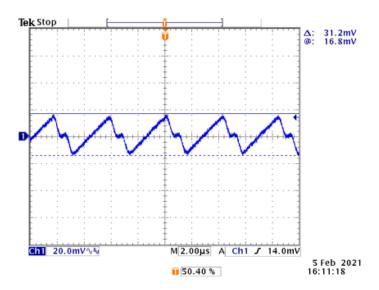
Figure 45. Typical Output Ripple Characteristic (V<sub>IN</sub> = 4.2VDC, I<sub>S</sub> = 100mA)
