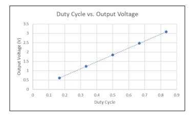
Figure 20. MAX38640A Duty Cycle Versus Output Voltage
