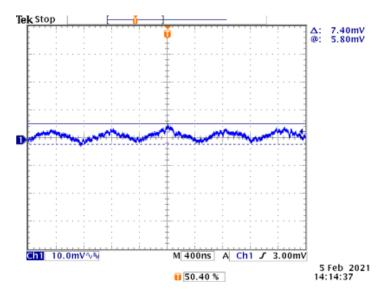
Figure 15. Typical Output Ripple Characteristic ( $V_{IN}$  = 4.2VDC,  $I_S$  = 100mA)
