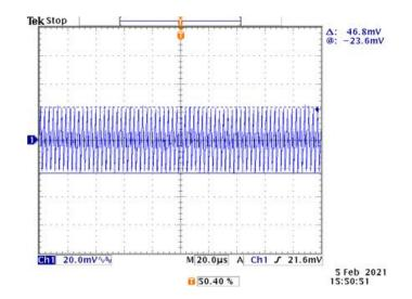
Figure 54. Typical Output Ripple Voltage ( $V_{IN}$  = 4.2V,  $I_S$  = 100mA)
