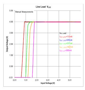
Figure 33. Line Load of the Analog 5V MAX20343H SMPS Circuit
