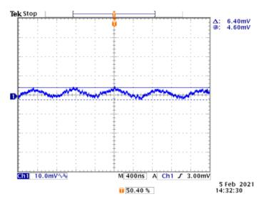
Figure 5. Typical Output Ripple Characteristic ( $V_{IN}$  = 4.2VDC,  $I_S$  = 100mA)
