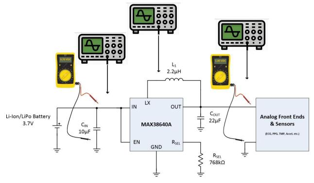
Figure 7. Troubleshooting the MAX38640A SMPS Circuit
