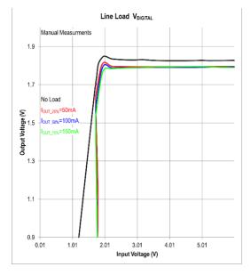
Figure 13. Line Load for the Digital MAX38640A SMPS Circuit
