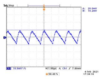
Figure 41. MAX20343H (5V) Output Ripple Waveform
