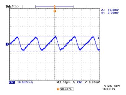
Figure 49. Typical Output Ripple Characteristic (V<sub>IN</sub> = 4.2VDC, I<sub>S</sub> = 100mA)
