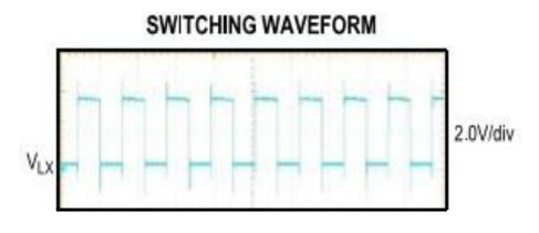
Figure 19. Typical MAX38640A VLX Waveform
