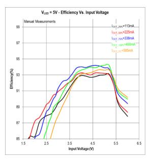
Figure 34. Efficiency of the Analog 5V MAX20343H SMPS Circuit
