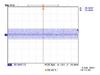
Figure 46. Typical Output Ripple Voltage (V<sub>IN</sub> = 4.2VDC, I<sub>S</sub> = 100mA)
