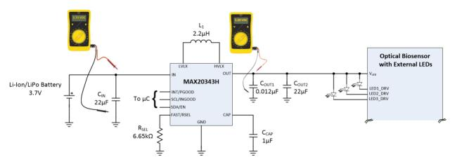
Figure 32. Analog 5VDC MAX20343H SMPS Circuit for Wearable Medical Applications
