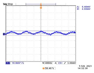
Figure 21. MAX38640A Output Ripple Waveform
