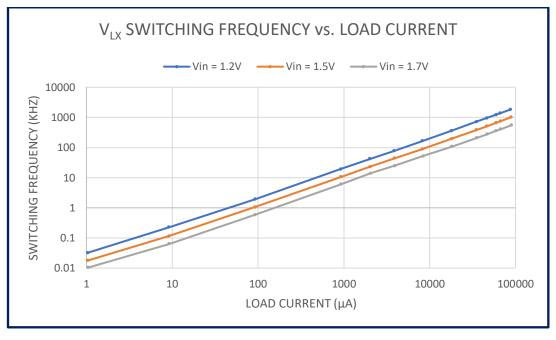
Figure 30: MAX17220 V<sub>LX</sub> Frequency vs. Load Current
