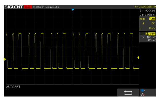
Figure 56. Typical MAX77642 LXA Waveform (SSB0 & SSB1  $I_{OUT}$  = 1.2mA; SSB2  $I_{OUT}$  = 126.1mA)
