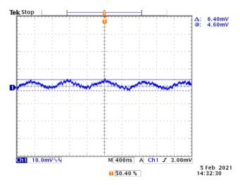
Figure 11. MAX38640A Output Ripple Waveform
