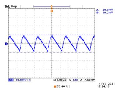
Figure 35. Typical Output Ripple Characteristic ( $V_{IN}$  = 4.2VDC,  $I_S$  = 100mA)
