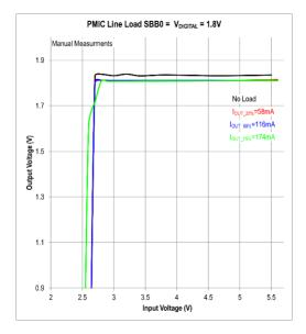
Figure 43. Line Load of the Digital 1.8V MAX77642 SMPS Circuit
