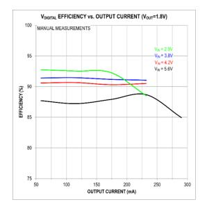
Figure 44. Efficiency of the Digital 1.8V MAX77642 SMPS Circuit
