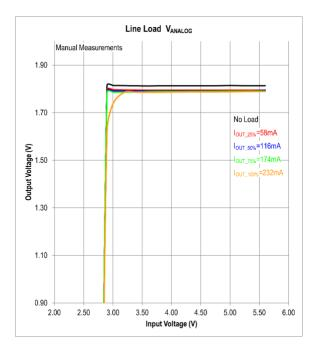
Figure 47. Line Load of the Analog 1.8V MAX77642 SMPS Circuit
