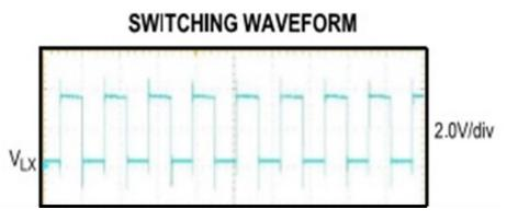
Figure 9. Typical MAX38640A VLX Waveform
