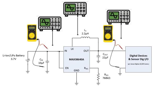
Figure 17. Troubleshooting the MAX38640A SMPS Circuit
