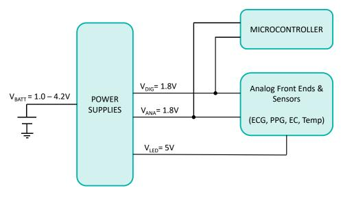
Figure 1. Typical Power Supply Configuration
