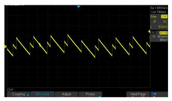
Figure 25. Typical Output Ripple Characteristic ( $V_{IN} = 1.5VDC$ ,  $I_S = 2mA$ )
