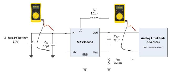
Figure 2. Analog 1.8VDC MAX38640A SMPS Circuit for Wearable/Healthcare Applications
