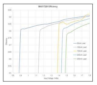
Figure 24. Efficiency of the Digital 1.8V MAX17220 SMPS Circuit
