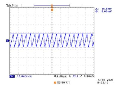
Figure 50. Typical Output Ripple Voltage (V<sub>IN</sub> = 4.2VDC, I<sub>S</sub> = 100mA)
