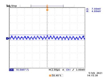
Figure 16: Typical Output Ripple Voltage (V<sub>IN</sub> = 4.2VDC, I<sub>S</sub> = 100mA)
