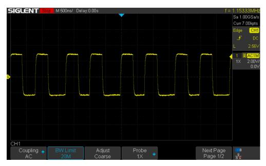
Figure 39. Typical MAX20343H HVLX Waveform with 125mA Load
