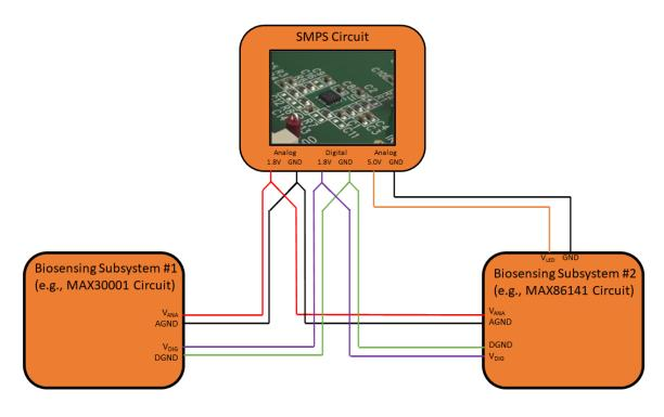
Figure 60. Power Supply "Star" Routing Topology
