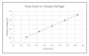
Figure 10. MAX38640A Duty Cycle Versus Output Voltage
