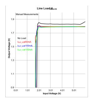
Figure 3. Line Load for Analog 1.8V MAX38640A SMPS Circuit
