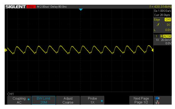
Figure 26: Typical Output Ripple Voltage ( $V_{IN} = 1.5VVDC$ ,  $I_S = 45mA$ )
