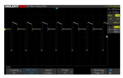
*Figure 29: Typical MAX17220 V<sub>LX</sub> Waveform with 45mA Load.*
