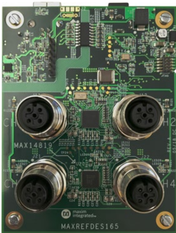
Figure 6. The MAXREFDES165# features the MAX14819.
