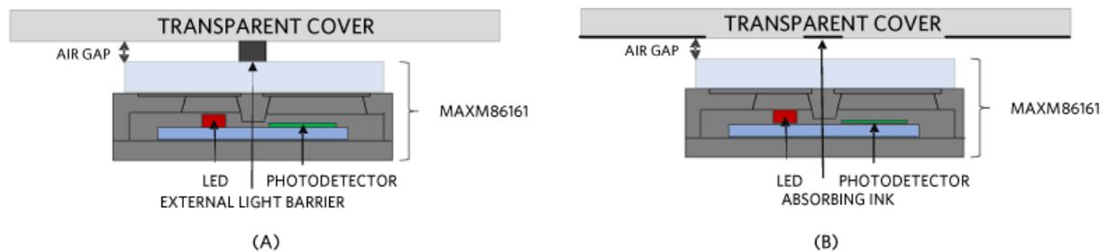
Figure 5. Light barriers (a) and inking (b).
