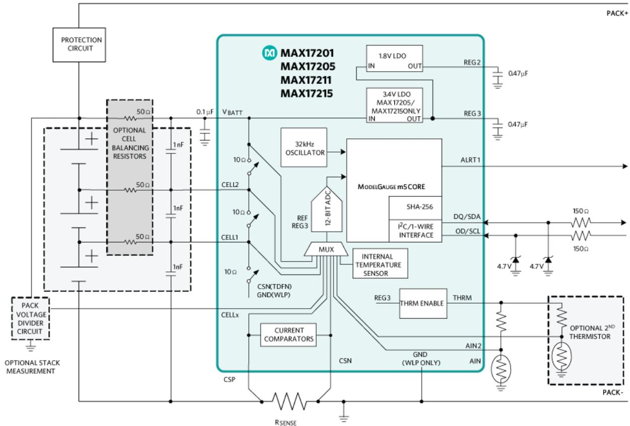
Figure 6. Block diagram of ICs implementing ModelGauge m5 EZ.
