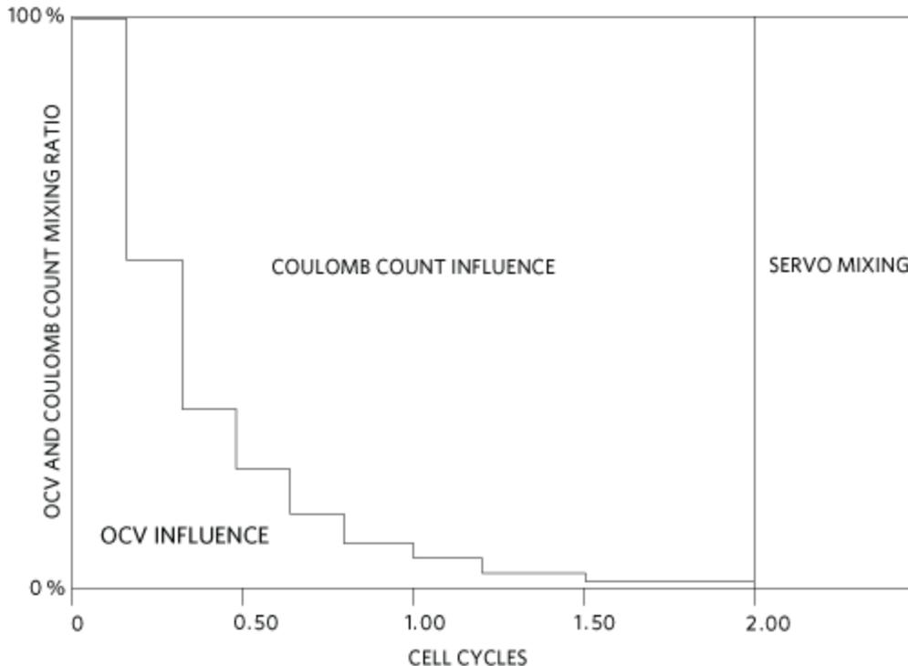
Figure 2. Voltage and coulomb count mixing.
