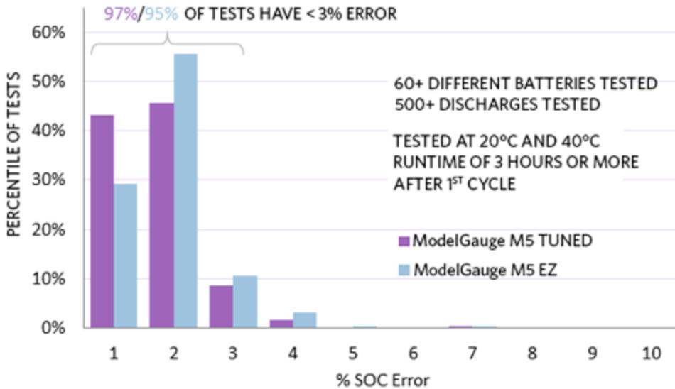
Figure 4. ModelGauge m5 EZ error compared to custom-tuned model.
