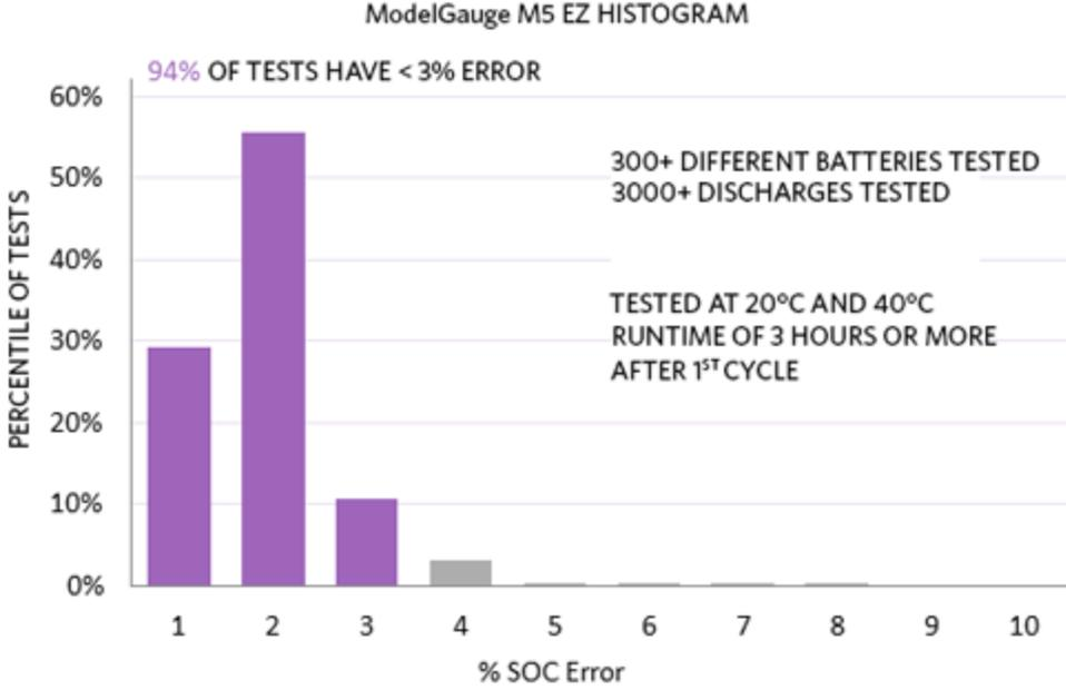
Figure 3. ModelGauge m5 EZ SOC error statistics on different batteries and discharges.
