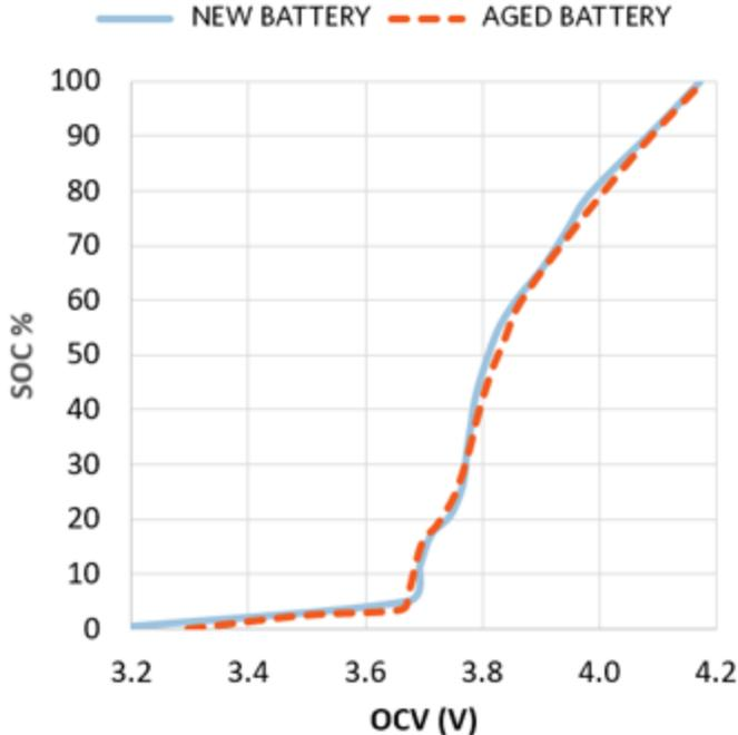
Figure 1. SOC% vs. OCV of a battery does not change with age.
