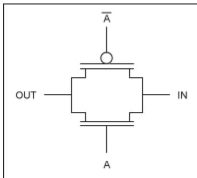
Figure 1. Schematic representation of a transmission gate.
