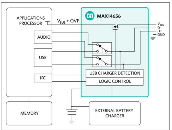
Figure 4. A smartphone application using the MAX14656 charger detector.
