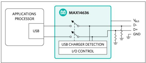
Figure 3. MAX14636 charger detector block diagram.
