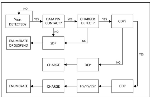
Figure 2. Summary of BC1.2 charger detection procedure.
