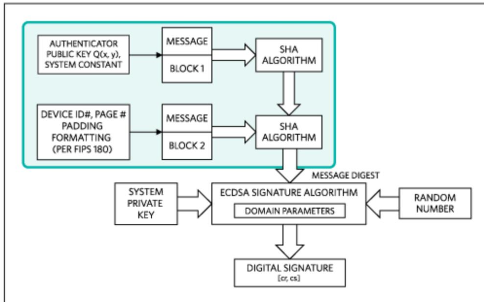
Figure 6. Certificate generation by a key-management system.
