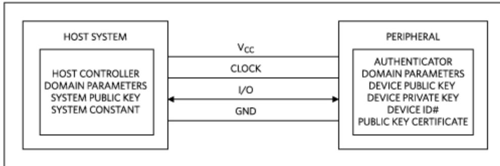
Figure 5. Hardware configuration of an ECDSA authentication system.
