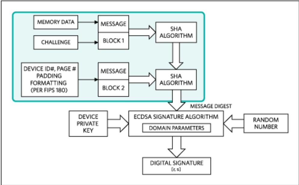
Figure 9. Signature computation performed by the authenticator.
