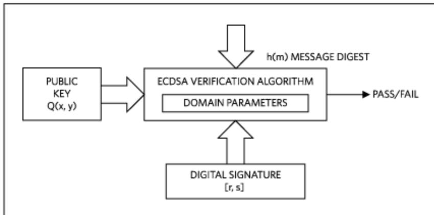
Figure 4. Signature verification process.
