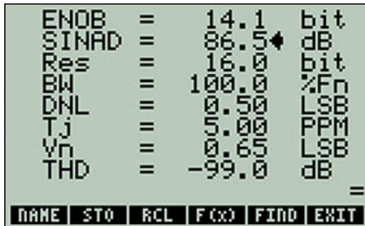
Figure 10. The MAX1162 is shown to have a SINAD of 86.5dB.
