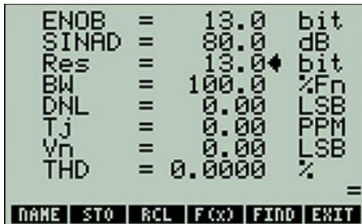
Figure 4. The ENOB Calculator determined that 13 bits of resolution are required in our example.
