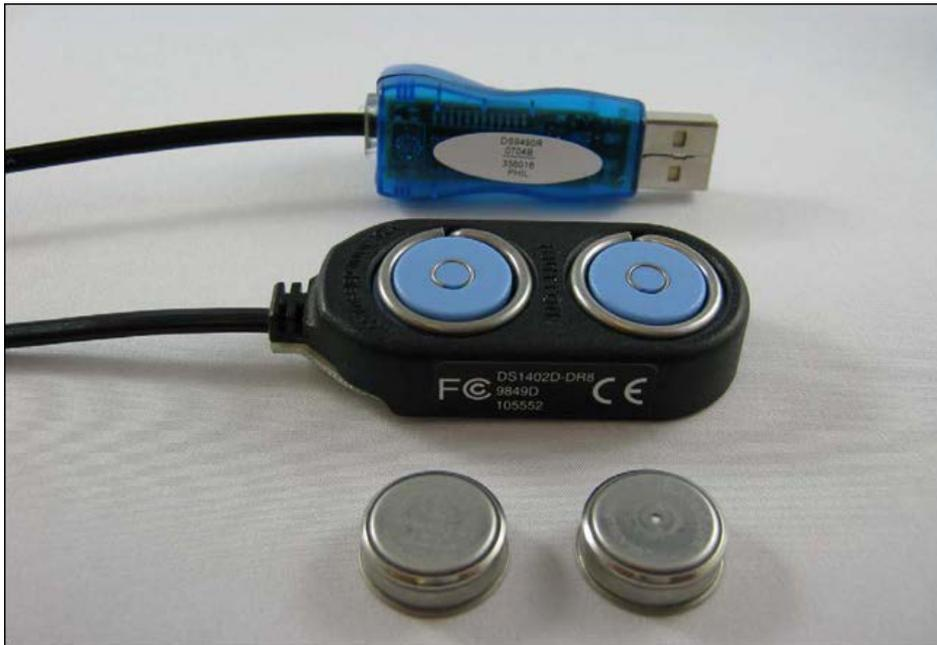
Figure 1. From front to back: logger iButtons, a Blue Dot™ receptor, a USB adapter.
