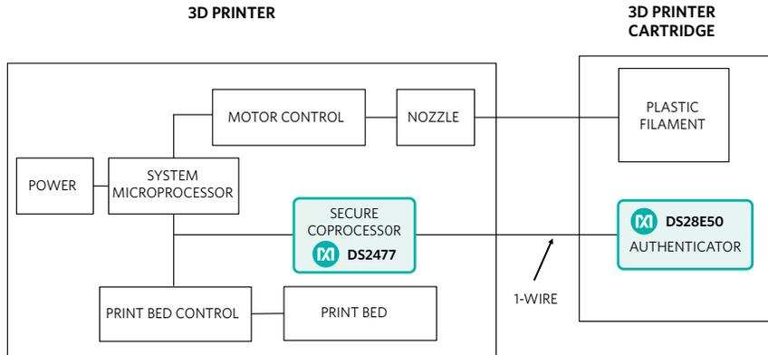
Figure 3. 3D printer cartridge authentication
