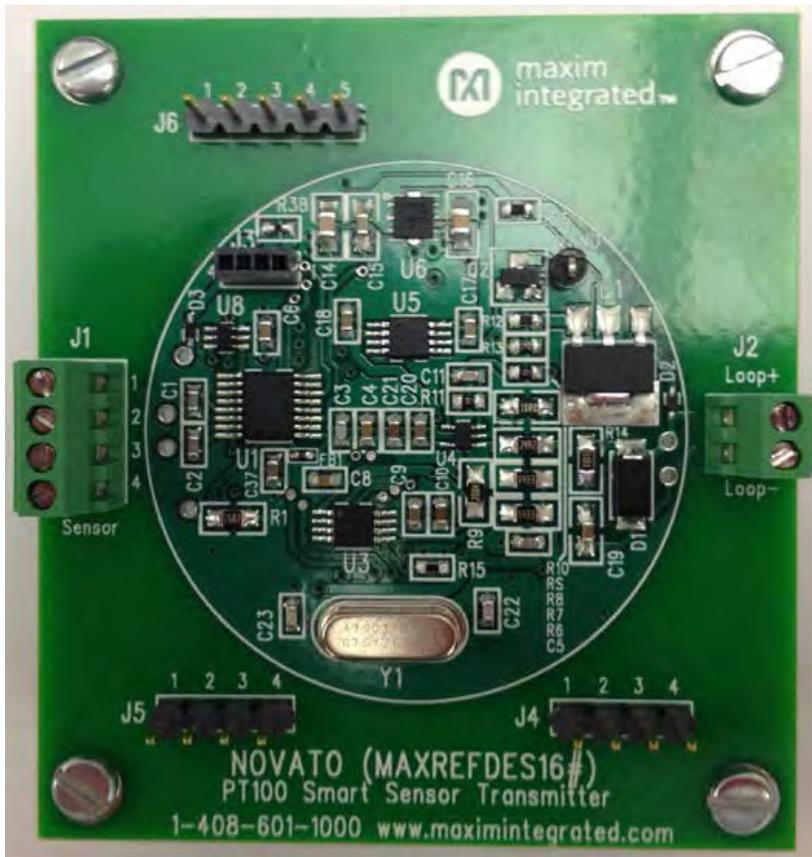
Figure 4. Novato smart sensor transmitter.
