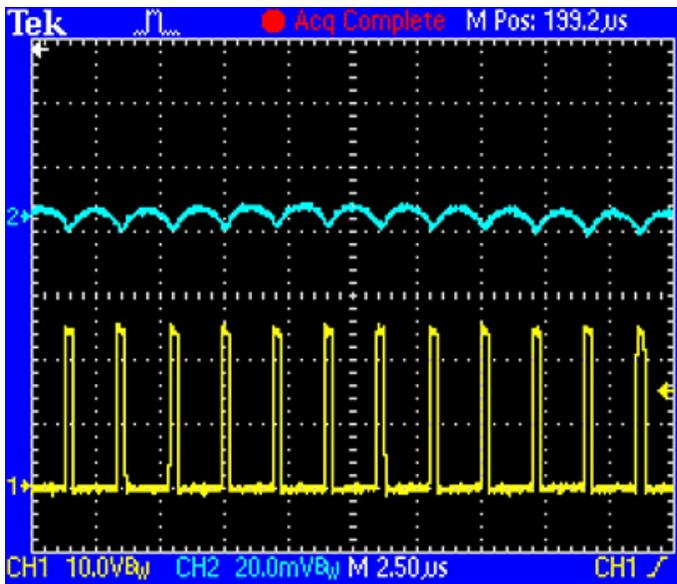
Figure 4. Output ripple at 300mA load.
