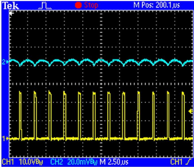
Figure 3. Output ripple at 0mA load.
