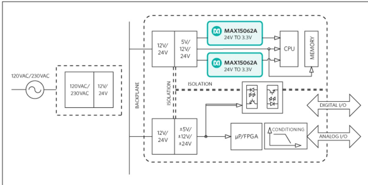
Figure 1. Typical industrial control power system diagram.
