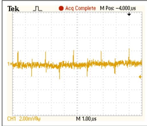
Figure 7. Noise at  $V_{OUT} = 15V$ ,  $I_{OUT} = 60mA$ .
