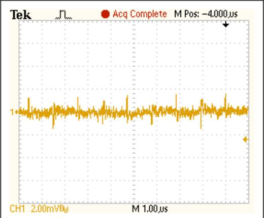
Figure 5. Noise at VOUT = 15V, IOUT = 0mA.
