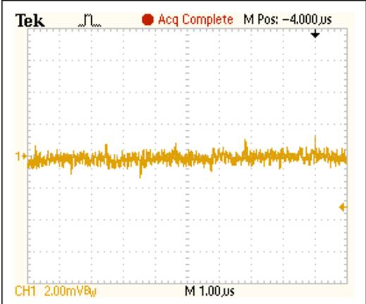
Figure 4. Noise at VOUT = 12V, IOUT = 0mA.
