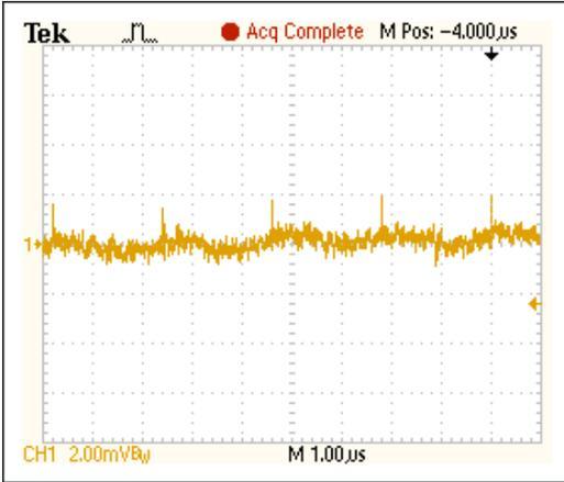
Figure 6. Noise at  $V_{OUT} = 12V$ ,  $I_{OUT} = 165mA$ .
