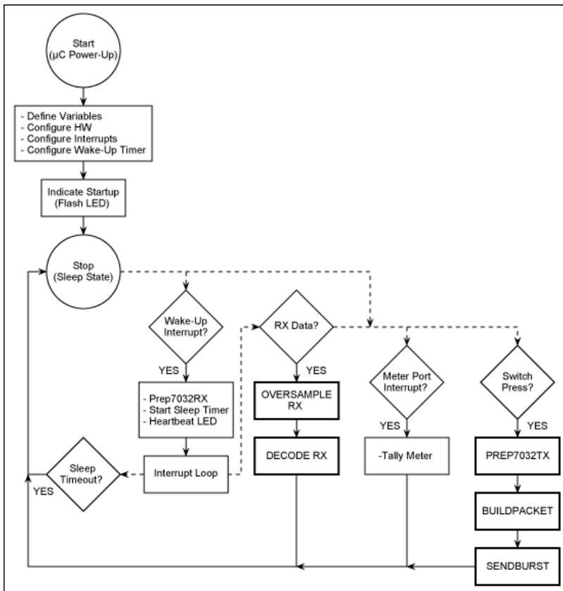
Figure 1. RF module functional operation.
