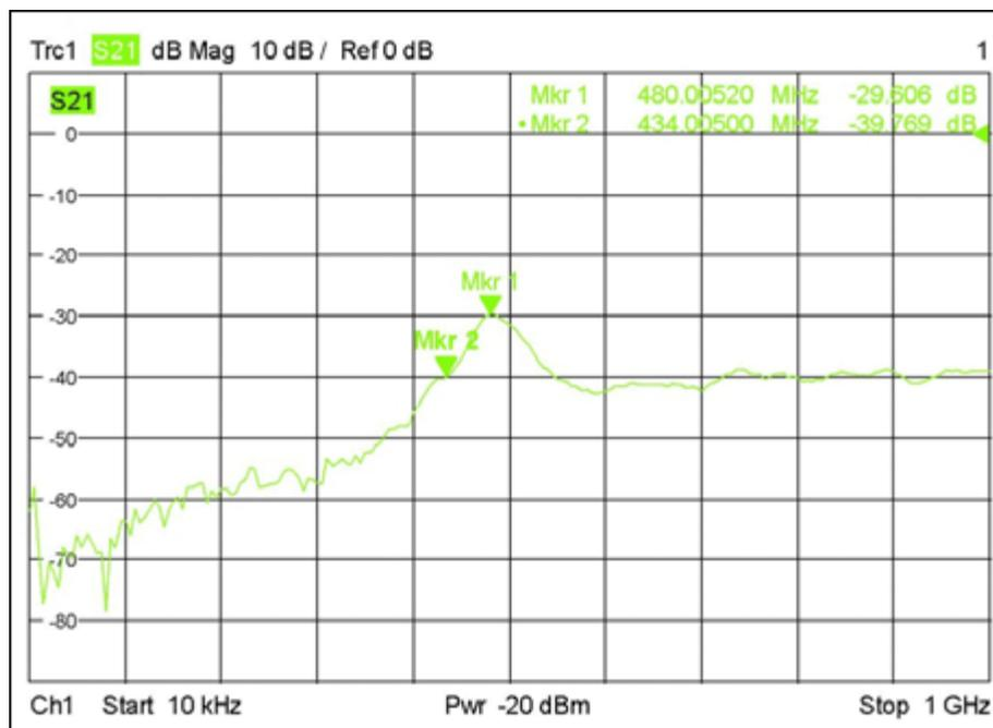
Figure 2. Tank circuit frequency before tuning.
