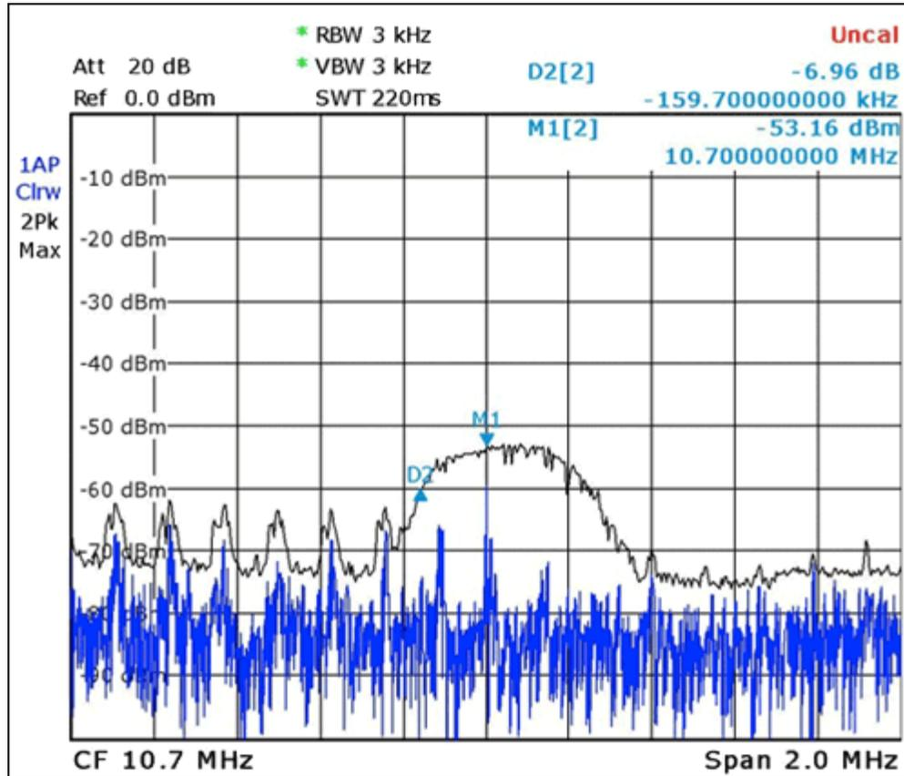
Figure 1. IF filter bandwidth, max-hold sweep.
