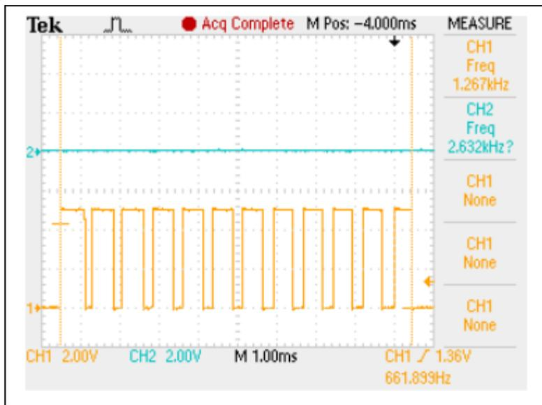
Rx data oscilloscope capture.
