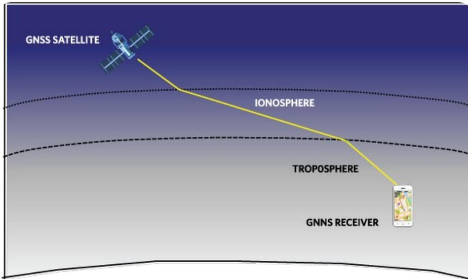
Figure 3. Ionosphere and Troposphere Atmospheric Delays Occur Between the GNSS Satellite and GNSS Receiver
