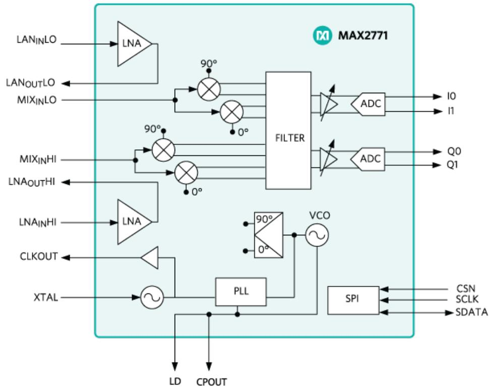
Figure 6. Multiband Universal GNSS Receiver
