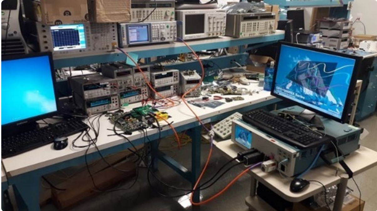
Figure 3. Bench setup with DPO72304SX digital phosphor oscilloscope.
