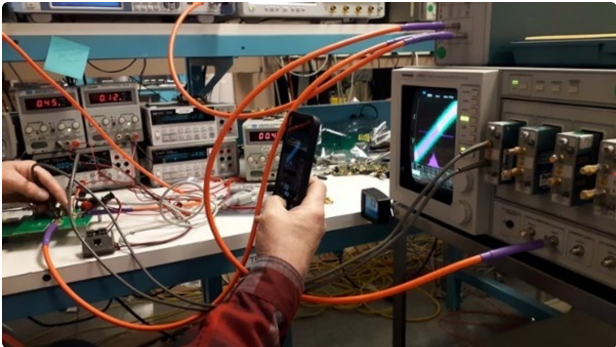
Figure 2. Test setup with TEK 11801C.
