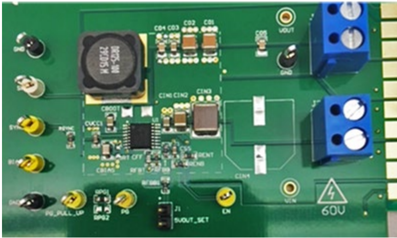
Figure 4b. Evaluation board of buck converter with simple internal compensation.
