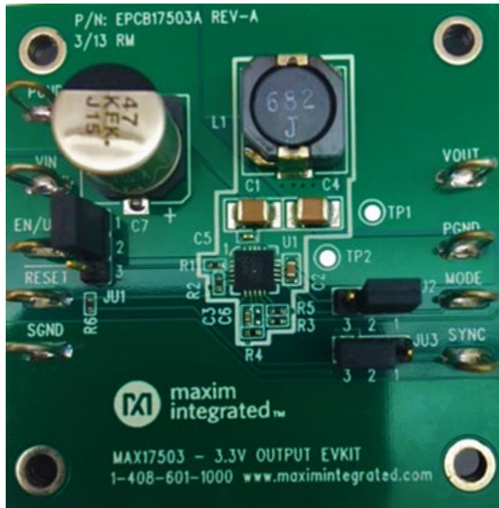
Figure 6b. Evaluation board of buck converter with wide-bandwidth internal compensation.
