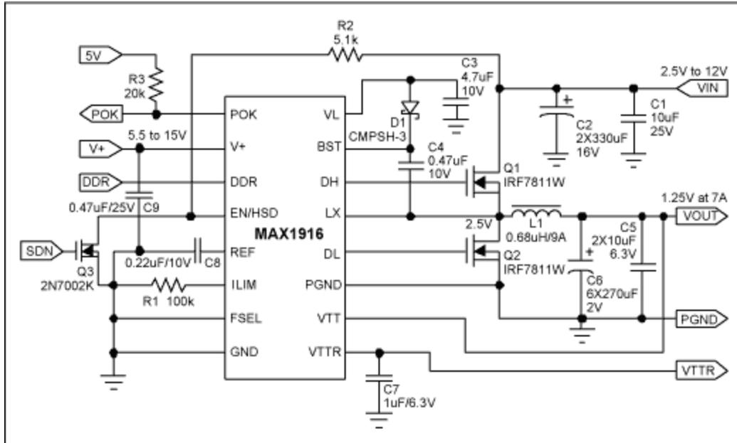
Figure 1. Schematic of 1.25V/7A VTT supply.
