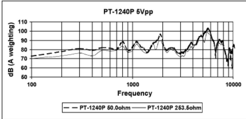
Figure 12. PT-1240P with 5V<sub>P-P</sub> excitation.
