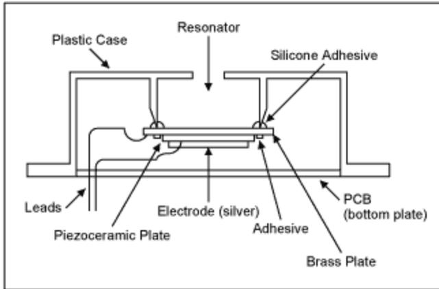
Figure 1. Cut-away view of audible PZT.
