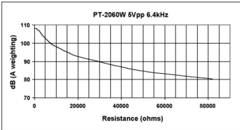
Figure 11. PT-2060W sound pressure vs. R<sub>source</sub>.
