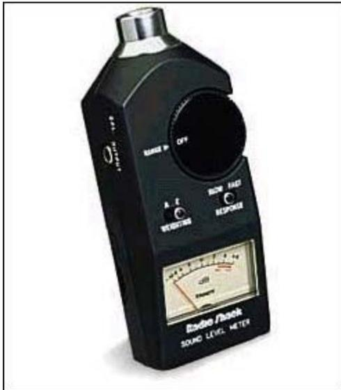
Figure 4. Radio Shack analog-display sound-level meter.
