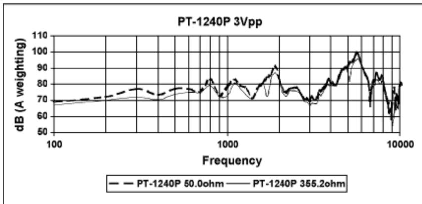
Figure 13. PT-1240P with 3V<sub>P-P</sub> excitation.
