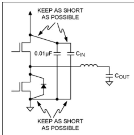
Figure 16. Placing a good ceramic  $0.01\mu\text{F}$  capacitor in parallel with the bulk input capacitance, and placing both capacitors directly across the MOSFETs (or catch diode) will help minimize ringing on the input supply due to the bulk capacitor's ESL.
