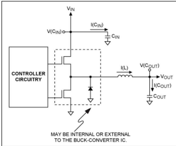
Figure 6. A typical buck converter circuit. Note that, depending on the buck converter used, the low-side MOSFET and or the catch diode may not be used.
