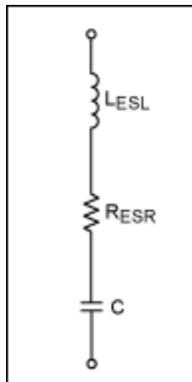
Figure 4. A model for capacitors used in buck converters.
