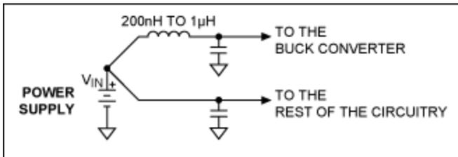
Figure 18. Adding some inductance in series with the buck converter will virtually eliminate the noise from the ESL of the input capacitor.
