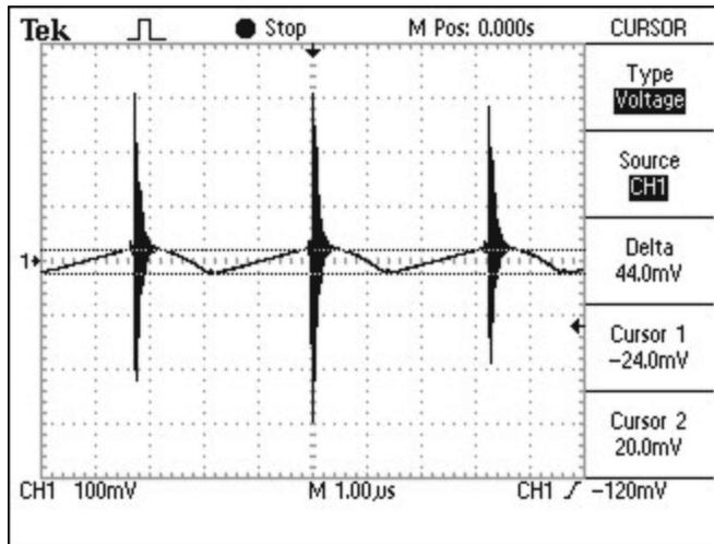
Figure 9. Shows a typical waveform of noise from finite input capacitance.
