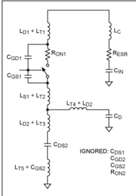
Figure 13. A simplified version of Figure 12 where some components are combined and trivial components are ignored.
