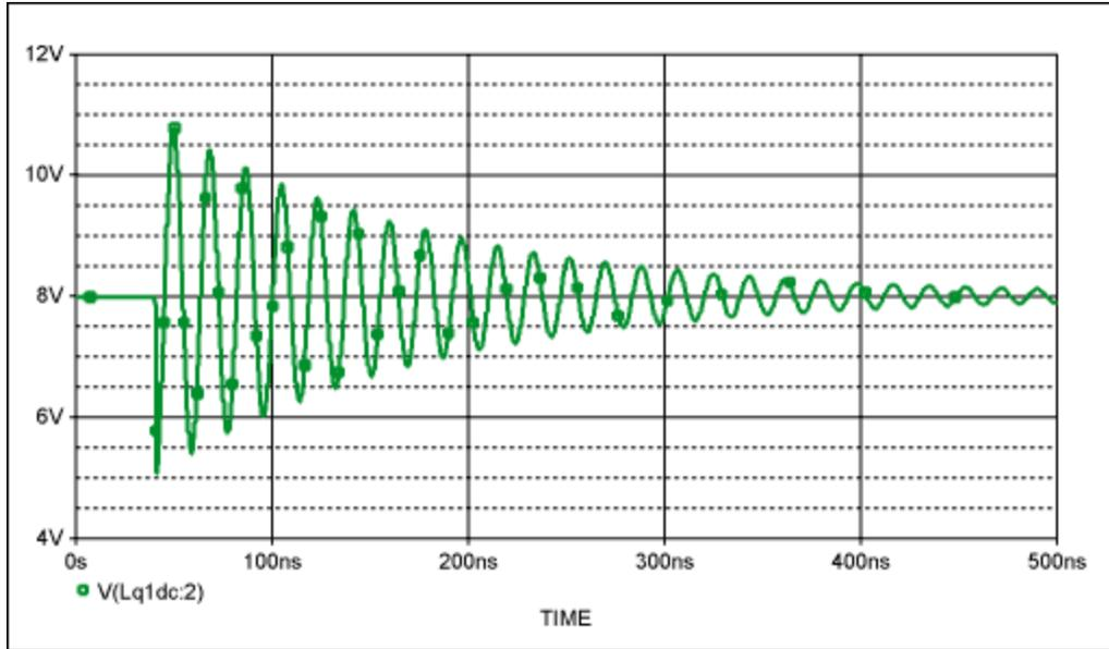
Figure 15. The ideal waveform of Figure 14 when the switch is closed. This waveform assumes that the input voltage (initial value of the capacitor) is 8V.
