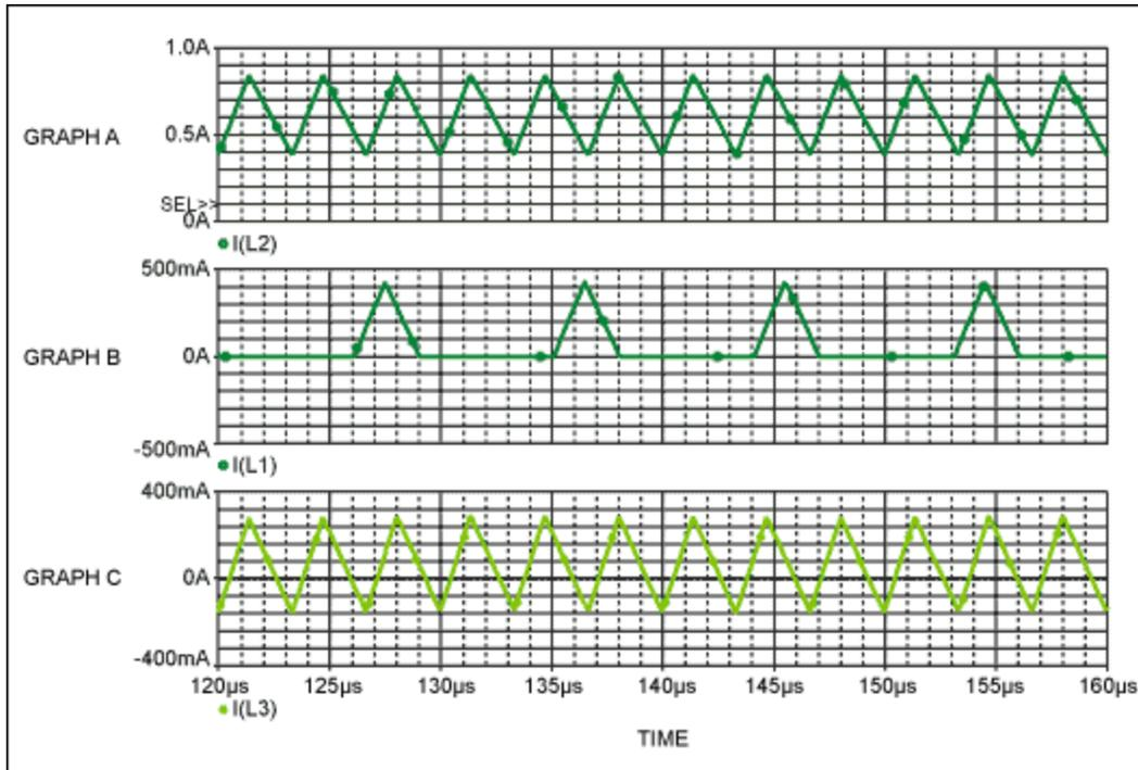
Figure 1. Three possible waveforms are shown for the current flowing through the inductor in a buck converter. Graph A shows continuous conduction operation where the current never drops below 0A. Graph B shows discontinuous conduction. Graph C shows continuous conduction where the current drops below 0A.
