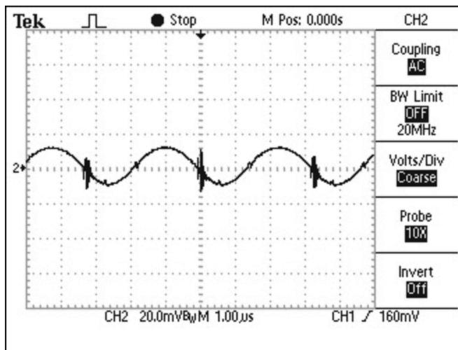
Figure 8. The noise on the output of a MAX1653EVKIT, using two 4.7µF ceramic capacitors. The measured peak-to-peak noise of 20mV agrees well with the calculated 18mV peak-to-peak.
