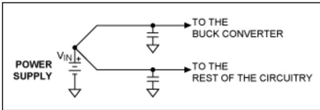
Figure 17. Separating the  $V_{IN}$  supply into two traces from the main power supply adds some trace inductance, which acts to filter the noise caused by the input capacitor's ESL.
