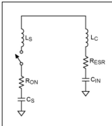
Figure 14. A further simplification of Figure 12. Technical accuracy of this drawing was sacrificed for simplicity.
