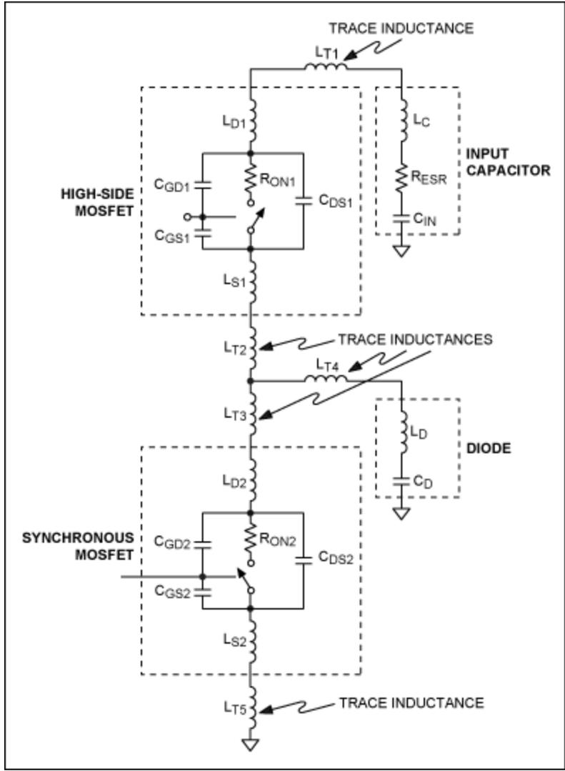
Figure 12. Shows the input side of a buck converter using the models developed earlier in this application note.
