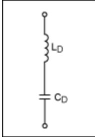
Figure 5. A model for reversed-biased diode used in a buck converter.
