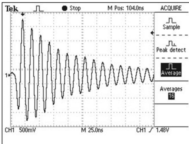
Figure 11. An expanded view of the high-frequency noise on the input supply of a buck converter.
