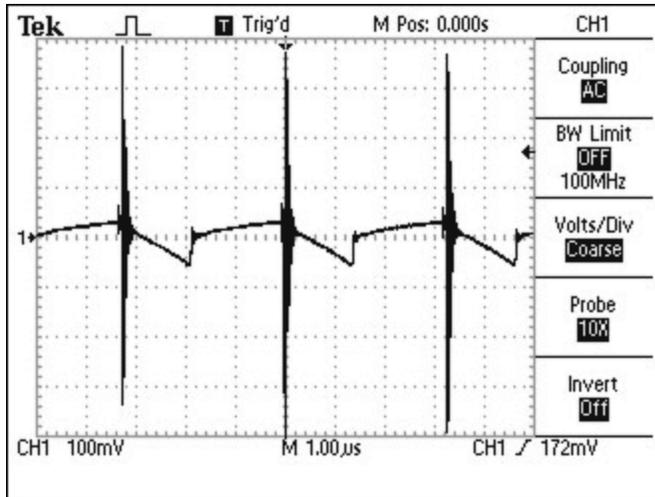
Figure 10. Shows the noise on the input due to the input capacitor's ESR.
