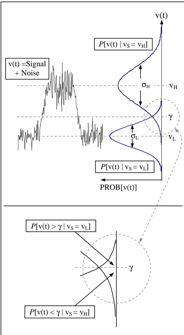
Figure 3. Probability of error for binary signaling
