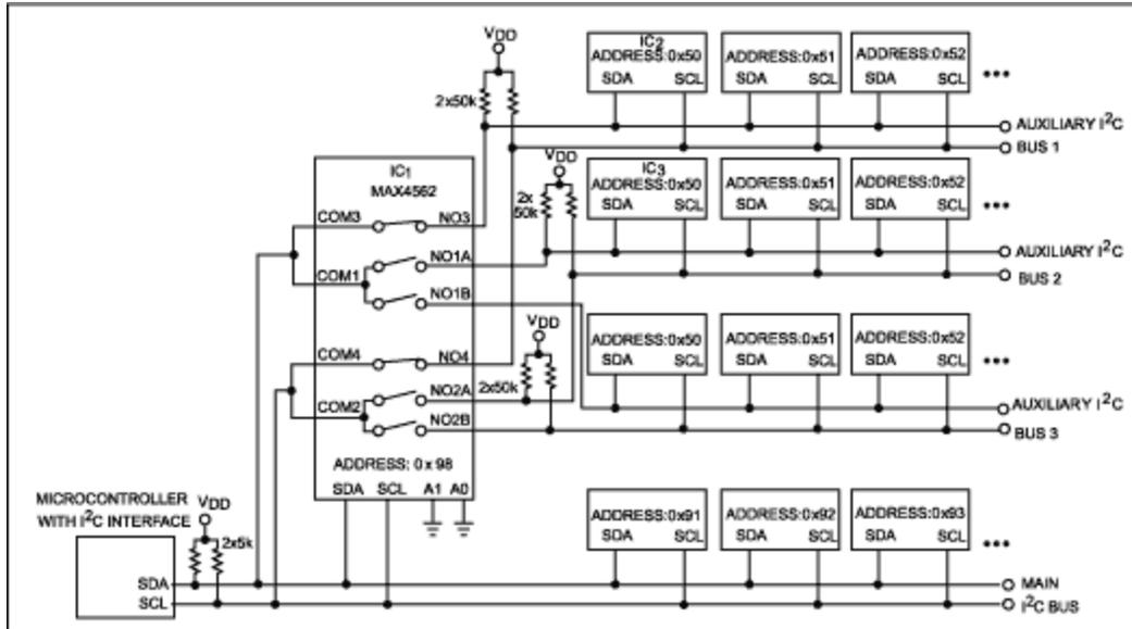
Figure 1. This I<sup>2</sup>C-controlled analog switch expands by three the number of devices connected to the bus.
