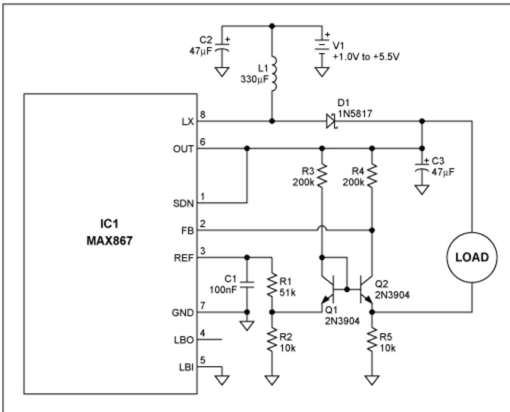
Figure 1. A low-cost feedback network (Q1, Q2, and associated resistors) improves the efficiency of this switchmode current source by a factor of six.
