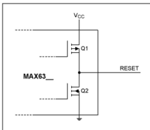
Figure 2. Push-pull output.
