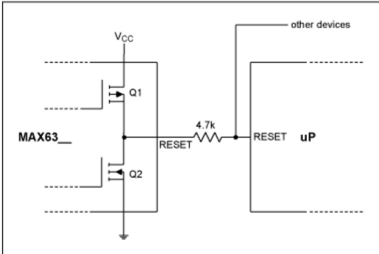
Figure 3. Interfacing to uPs with bi-directional reset.
