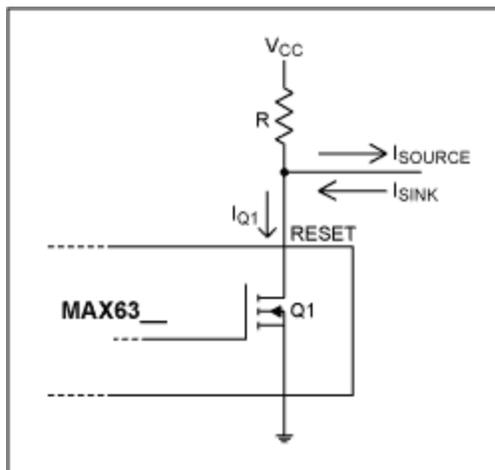
Figure 1. Open-drain output.
