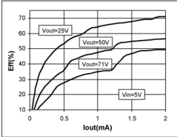
Figure 4. Efficiency curves.
