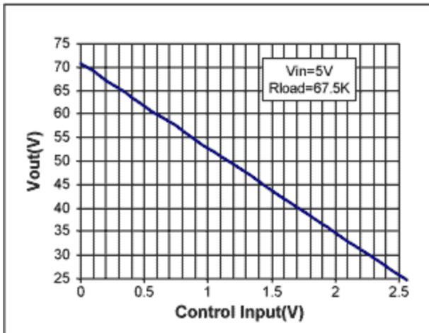
Figure 3. Measured output voltage vs. control input voltage.
