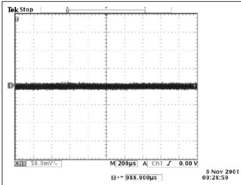
Figure 6. Output voltage ripple.  $V_{out}=71V$ ,  $I_{out}=1mA$ . With  $10\mu F$  electrolytic capacitor added in parallel to the  $1\mu F$  output capacitor. Vertical:  $50mV/div$ . Horizontal:  $200\mu s/div$ .
