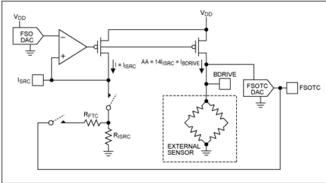
Figure 3a. Sensor-bridge excitation circuit.
