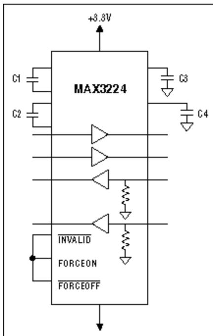
Figure 7. By connecting the ForceOn and ForceOff\* inputs to the Invalid\* outputs, an Autoshtutdown Plus part can be made to behave like an Autoshtutdown part.
