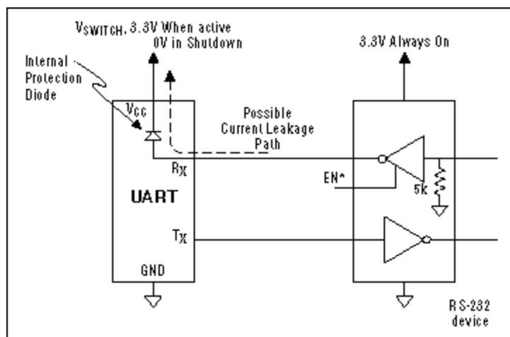
Figure 8. Some Maxim RS-232 devices have EN\* pins that allow the receivers to go into high-Z mode, so that the receivers won't forward-bias parts whose power supplies have been shut down to save
