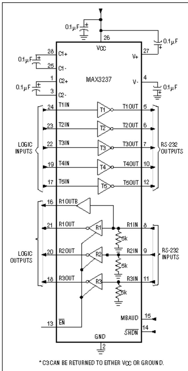
Figure 1. The MAX3237 has a pin labeled MBAUD that allows it to switch between RS-232-compliant
