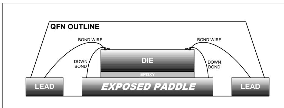
Figure 1. Internal Connection to the Exposed Paddle
