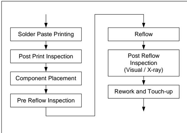
Figure 8: Board Mounting Process Flow (Reference [5](#))
