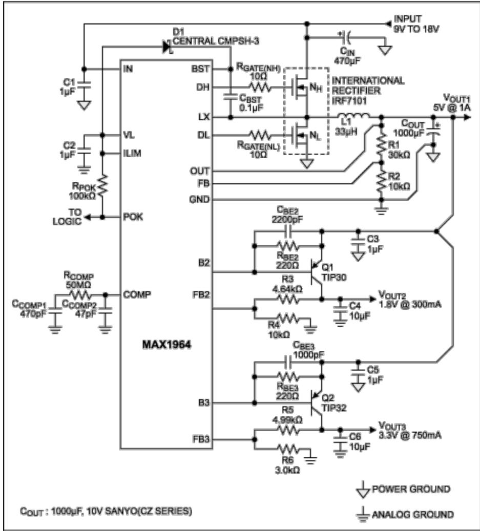
Figure 1. MAX1964 schematic.
