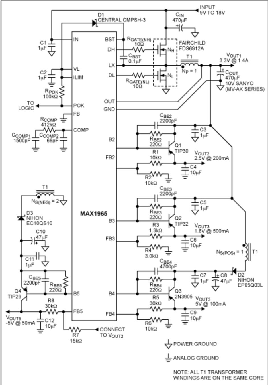
Figure 3. MAX1965 schematic.
