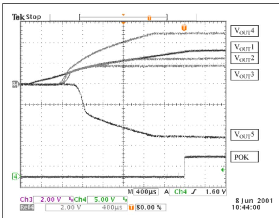
Figure 4. Output tracking sequence (from top trace down: V<sub>OUT4</sub>, V<sub>OUT1</sub>, V<sub>OUT2</sub>, V<sub>OUT3</sub>, V<sub>OUT5</sub>, and POK).
