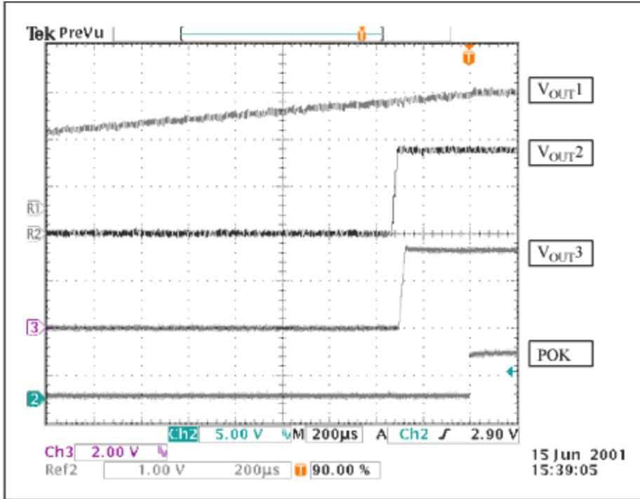
Figure 2. Output staggering sequence (from top trace down: V<sub>OUT1</sub>, V<sub>OUT2</sub>, V<sub>OUT3</sub>, and POK).
