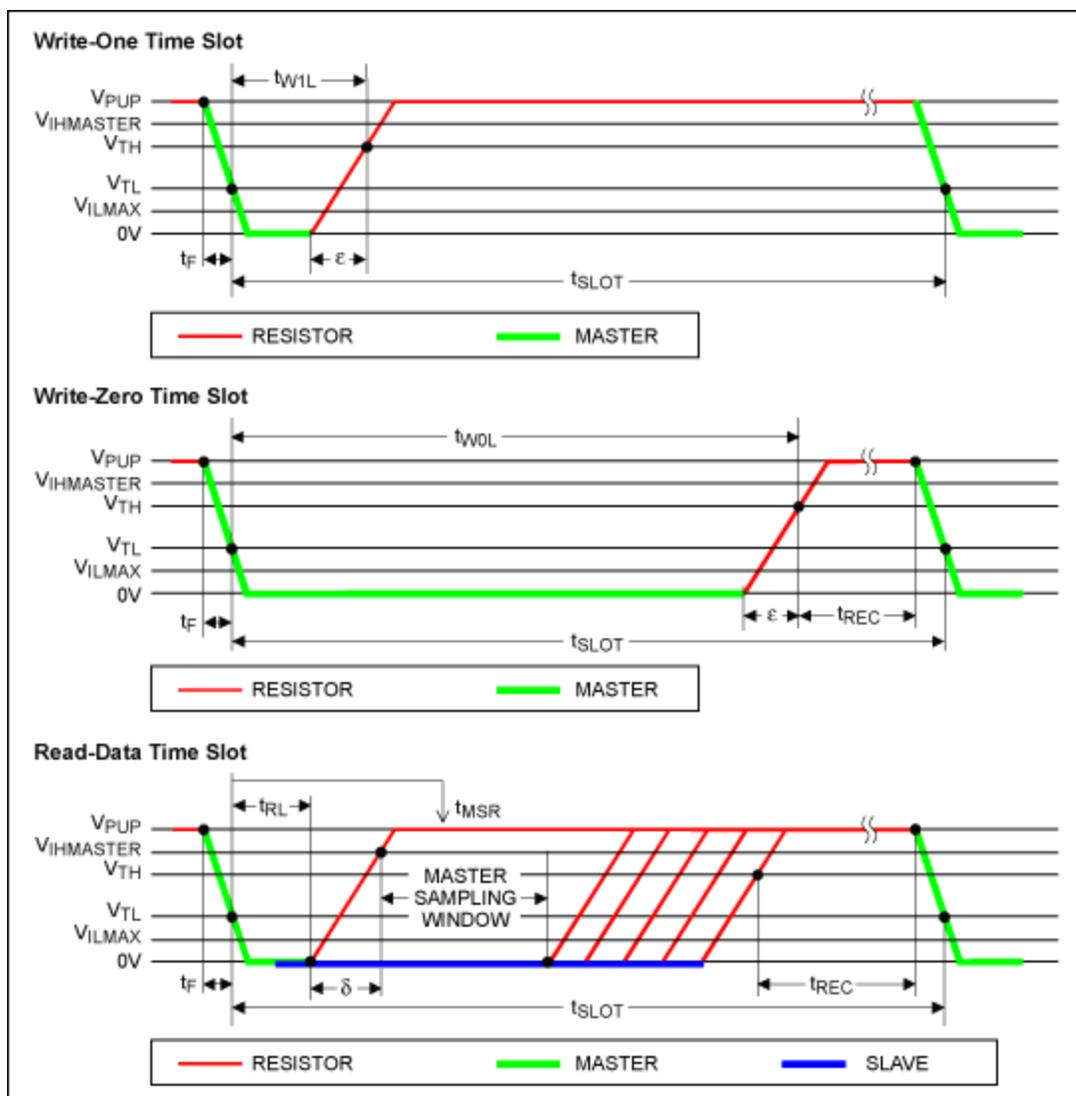
Figure 2. Read/write timing diagram.
