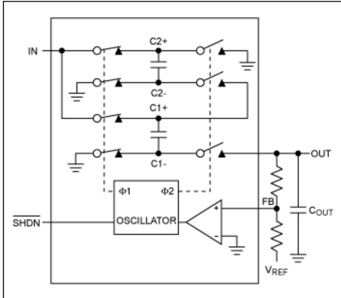
Figure 5. Internal components illustrate the operation of this regulated charge-pump inverter (MAX868).
