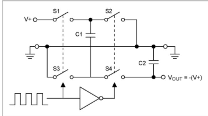
Figure 1. These essential components illustrate the mechanics of charge-pump operation.
