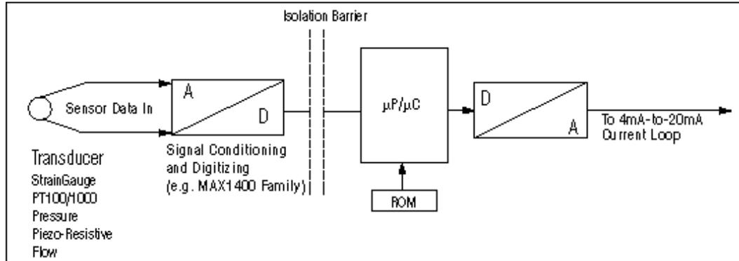
Figure 1. The inclusion of  $\mu\text{P}/\mu\text{C}$  intelligence makes this circuit a "smart" 4–20mA transmitter.
