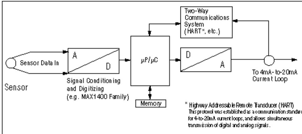
Figure 2. The association of  $\mu P/\mu C$  intelligence with the sensor produces an "intelligent" 4–20mA transmitter.
