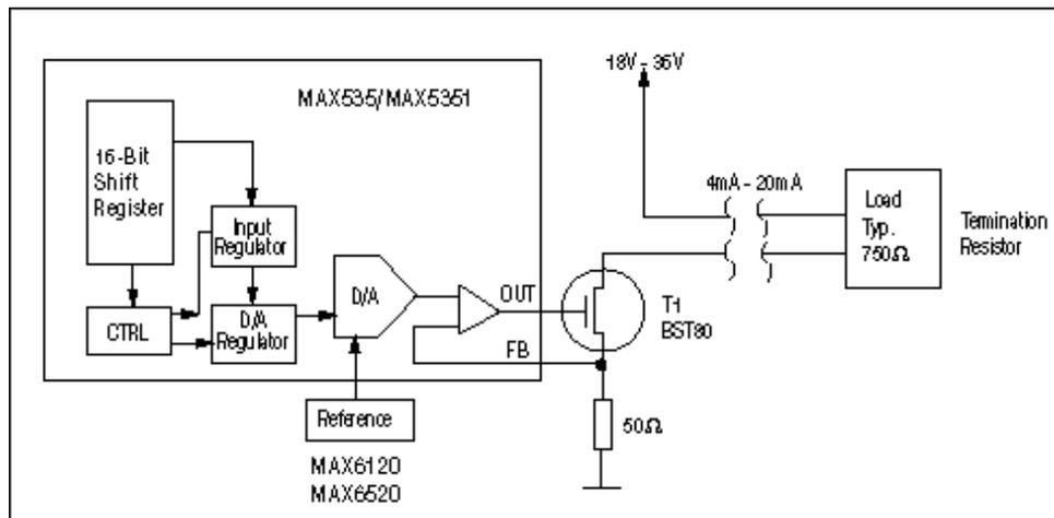
Figure 3. This simple, digitally adjustable 4–20mA current loop is suitable for transmission over moderate distances.
