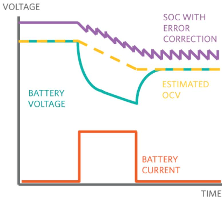
Figure 4. Accurate fuel gauging with ModelGauge M5.
