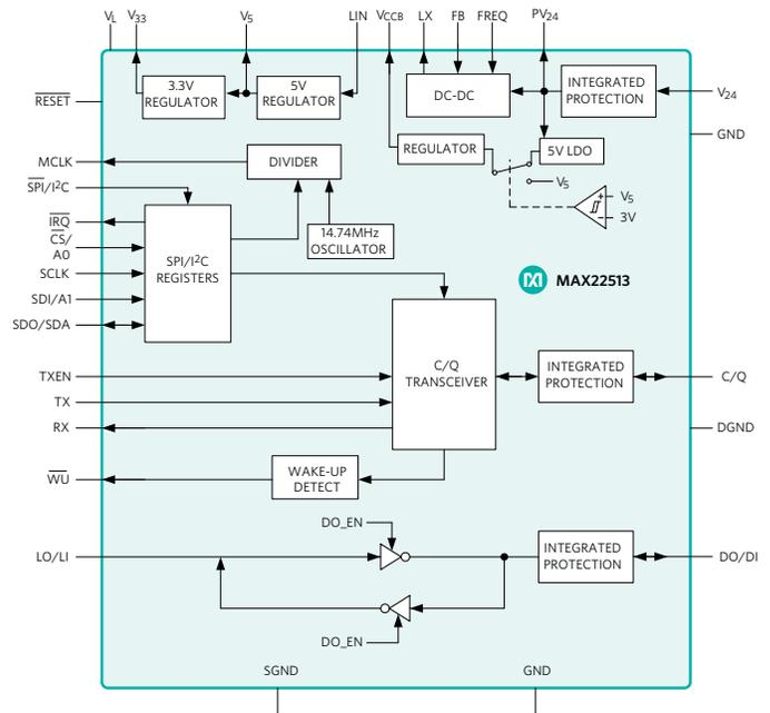
Figure 7. MAX22513 Dual-Channel IO-Link Transceiver
