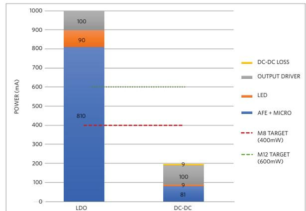
Figure 5. Power Reduction Using a Buck Converter vs. LDO
