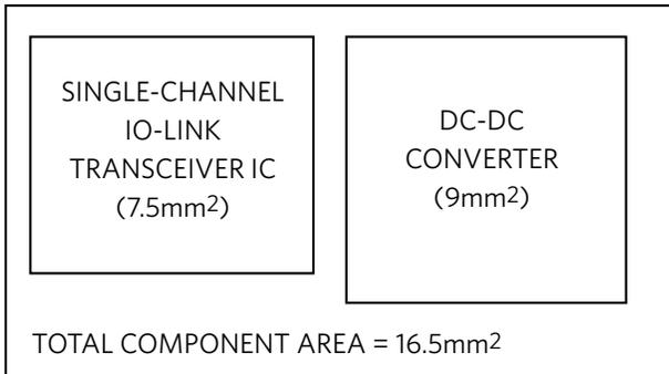
Figure 6. Typical IO-Link Transceiver Solution
