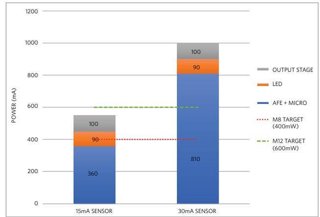
Figure 4. Power Budget (mW) for Typical Inductive Sensors
