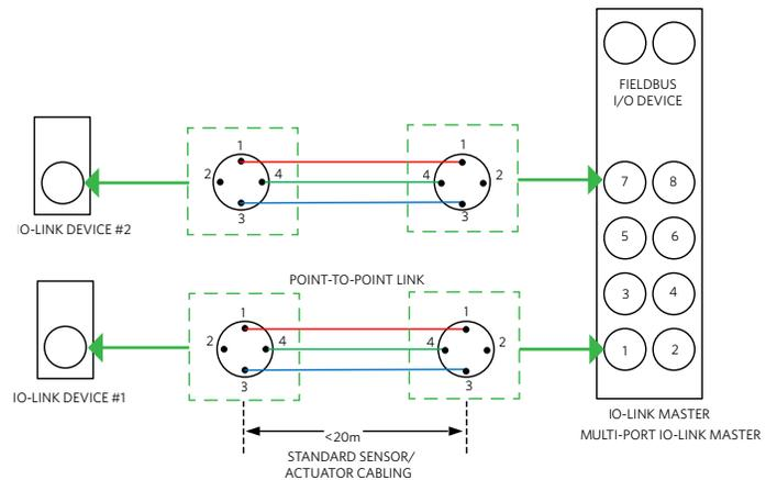
Figure 2. IO-Link Master/Device Interface
