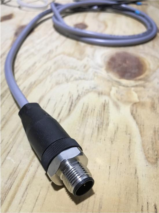
Figure 3. M12 Sensor Connector
