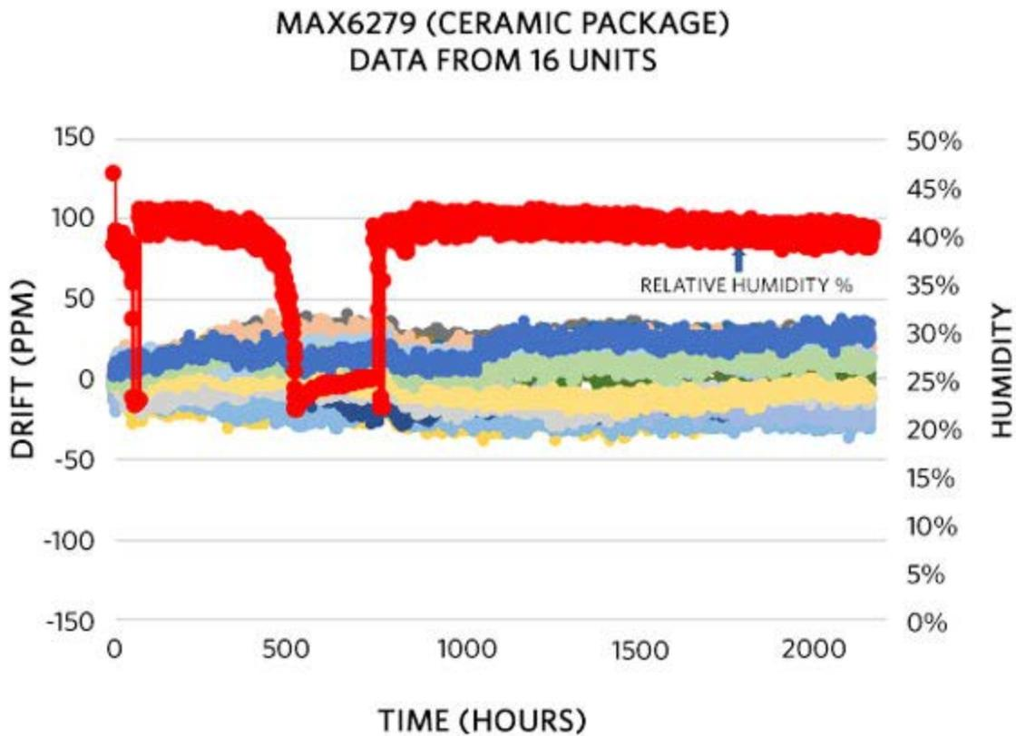
Figure 11. MAX6279 ceramic test chip LTD with regard to relative humidity.
