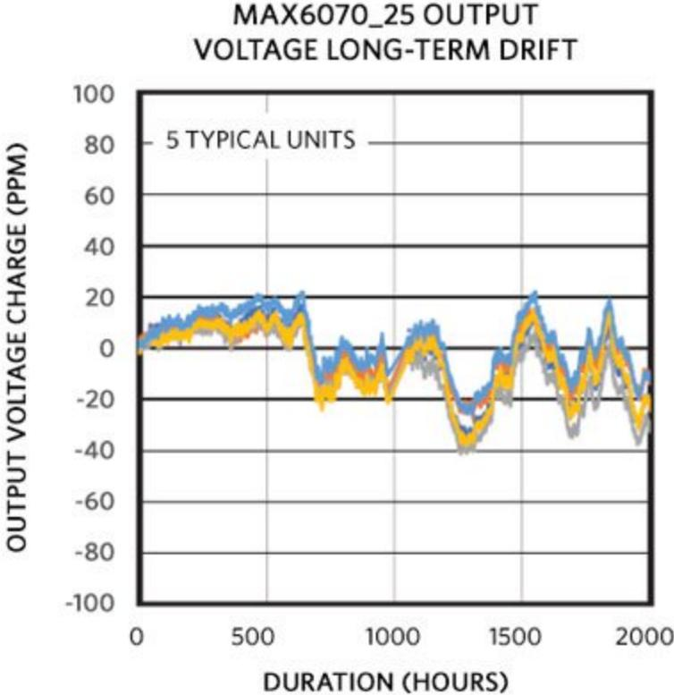
Figure 1. LTD plot for SOT-23 package.
