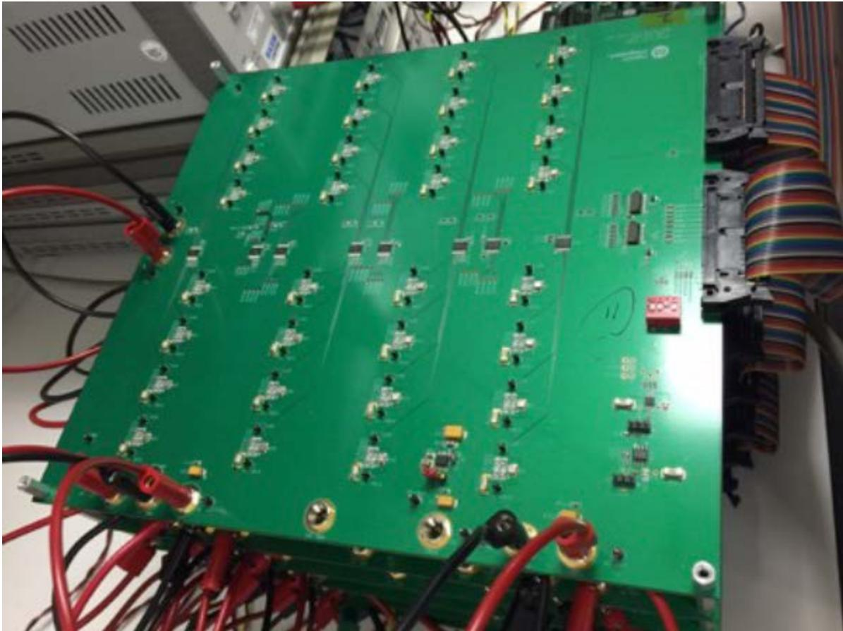
*Figure 4. Multisite voltage reference PCB.*
