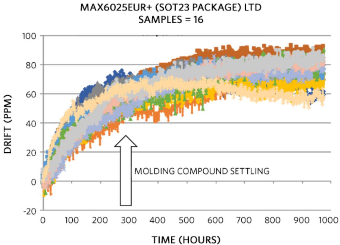
Figure 7. Package compound settles during the first 200-300 hours.
