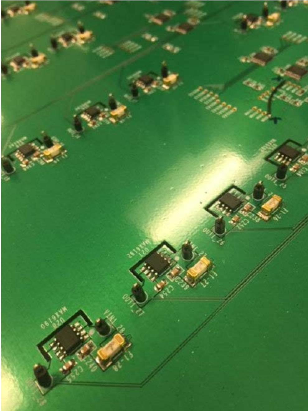
Figure 3. Three-side cut-out "slotting" to relieve solder joint stress.
