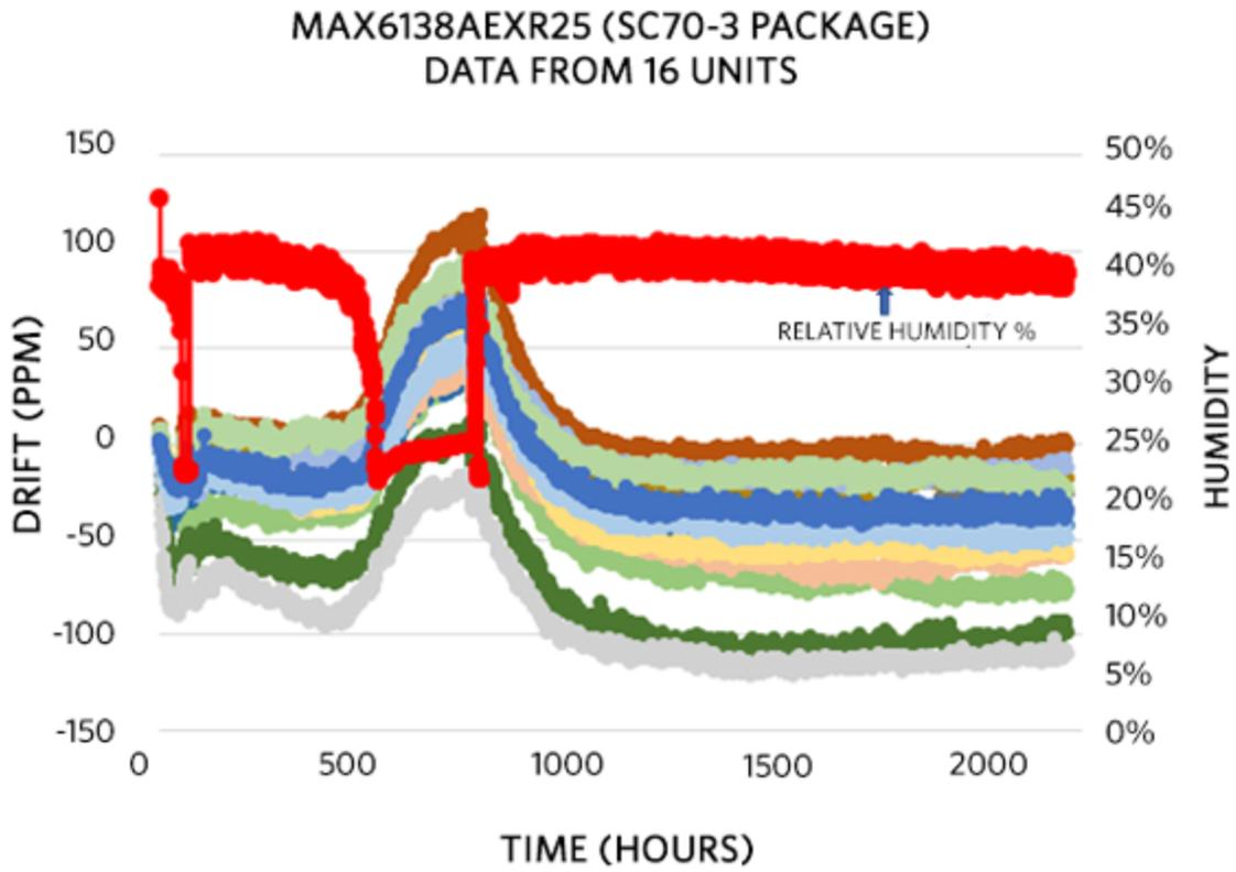
Figure 10. MAX6138AEXR25 (SC70-3 plastic package); LTD with regard to relative humidity.
