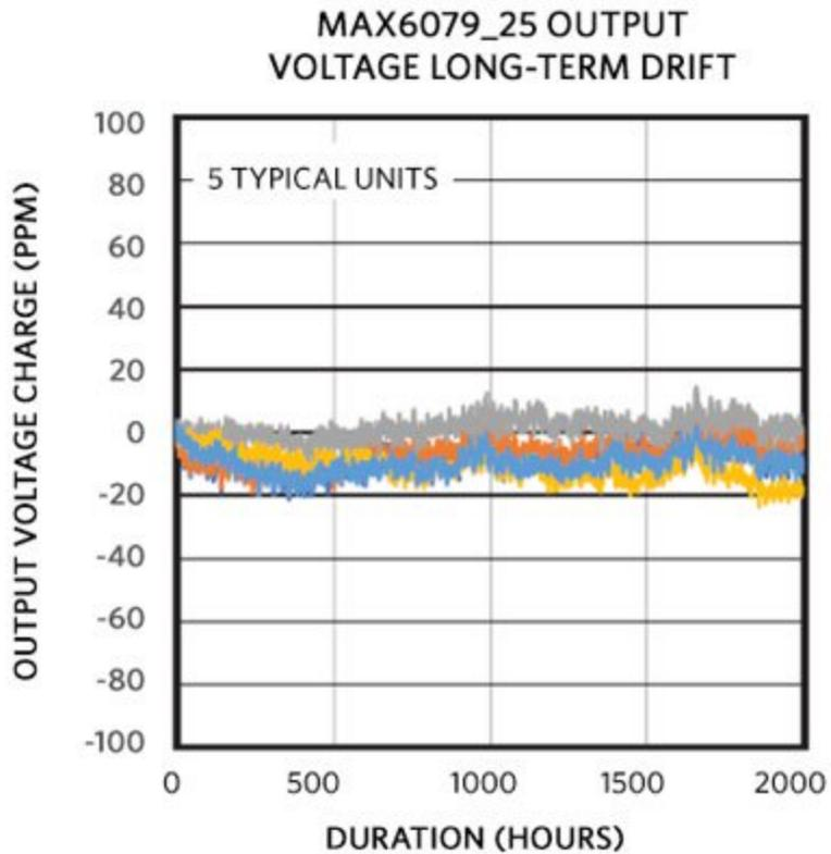
Figure 2. LTD plot for ceramic package.
