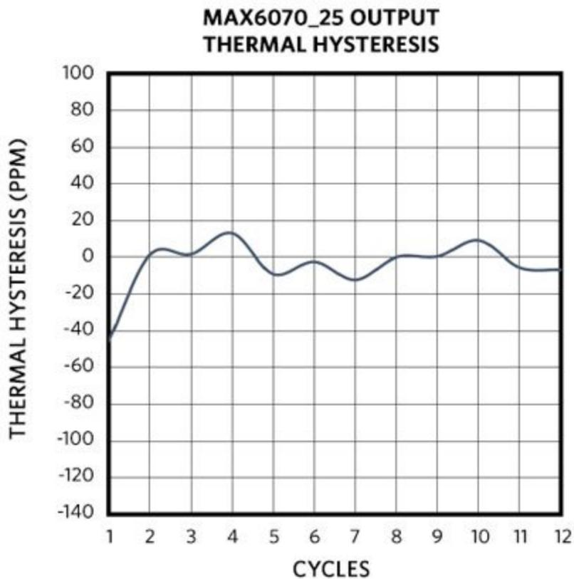
Figure 9. Typical thermal hysteresis plot.
