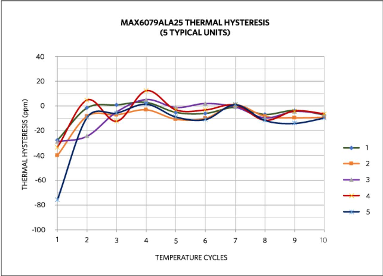
Figure 1. Five units of MAX6079 measured through 10 temperature cycles.
