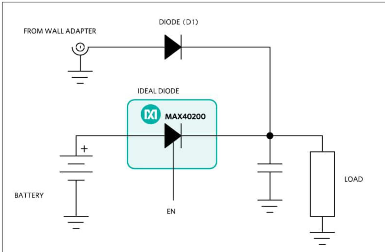
Figure 3. Diode ORing circuit
