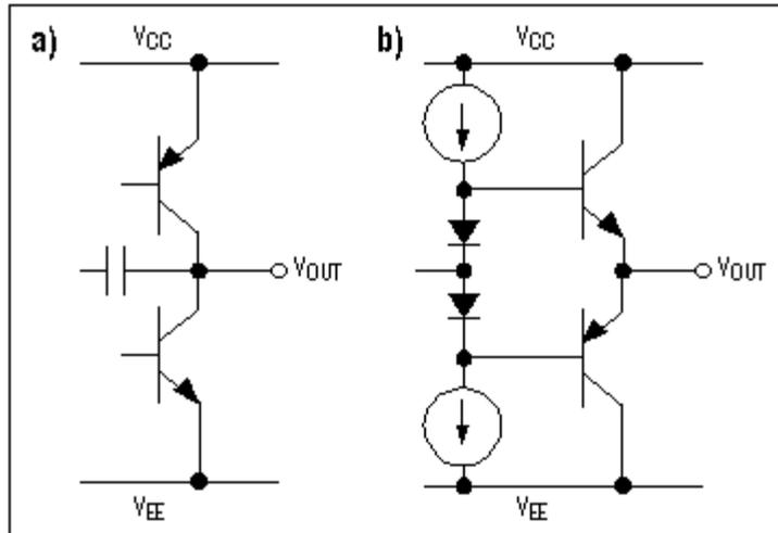
Figure 5. A rail-to-rail output stage (a) has a common-emitter configuration, while a standard output stage (b) has an emitter-follower configuration.
