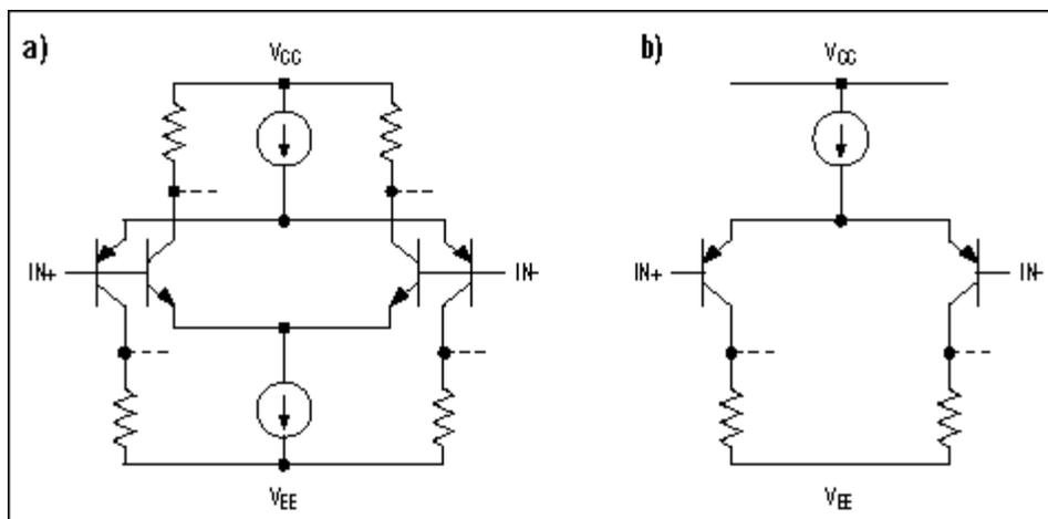
Figure 1. A rail-to-rail input stage (a) has two differential pairs, while a standard ground-sensing input stage (b) has only one.
