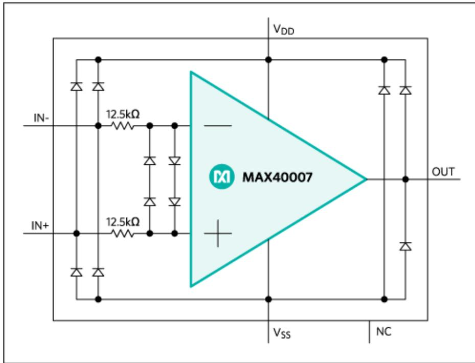
Figure 1. The MAX40007 nanoPower op amp is available in ultra-tiny WLP and SOT23 packages.
