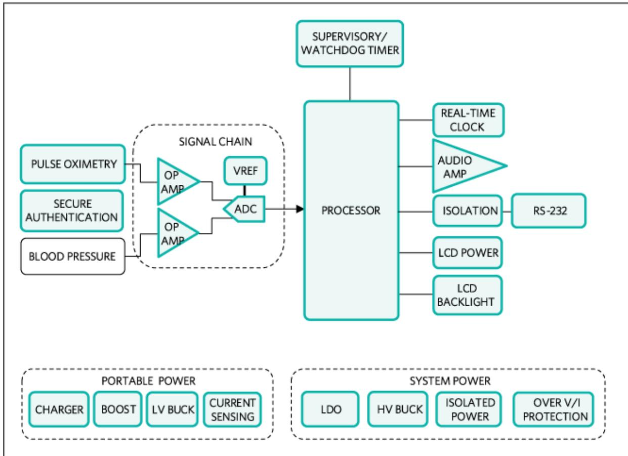
Figure 2. Block diagram of an example patient monitoring design, showing key components inside.
