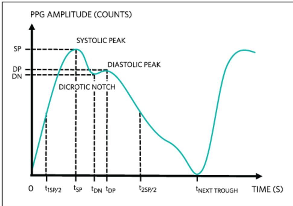
Figure 2. Typical PPG waveform.
