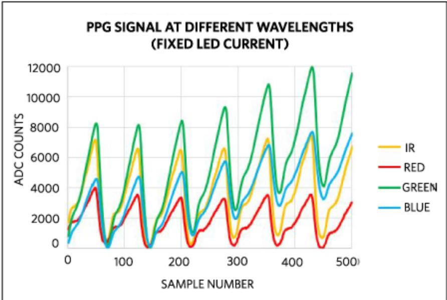
Figure 1. Backscattered light received by the photodetector of a PPG.
